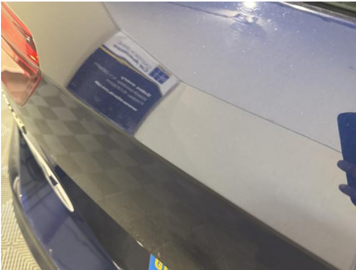
11: Boot Lid Dented Over 2 UpTo 10mm
