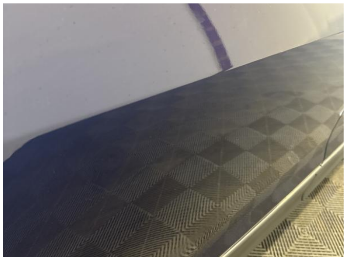
14: Door osr Dented Over 30mm
