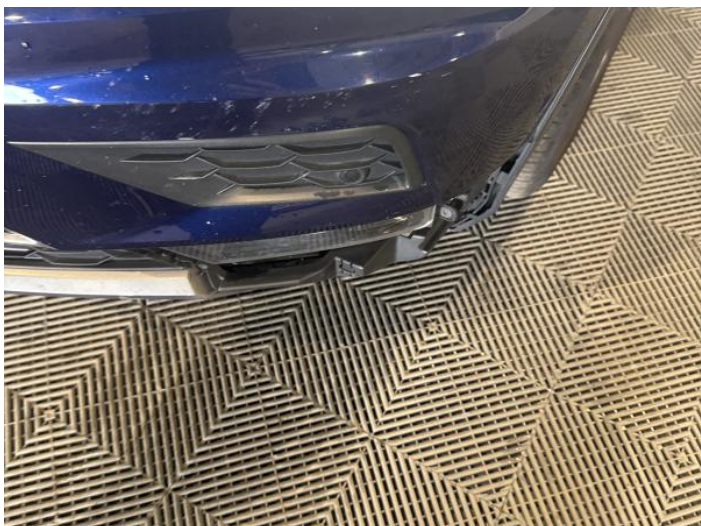
3: Bumper Front Moulding Broken Replace
