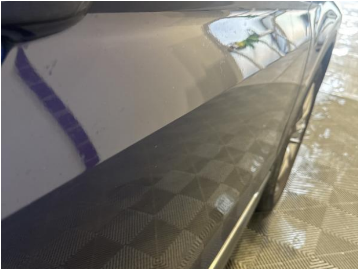
15: Door osf Dented Over 2 UpTo 10mm
