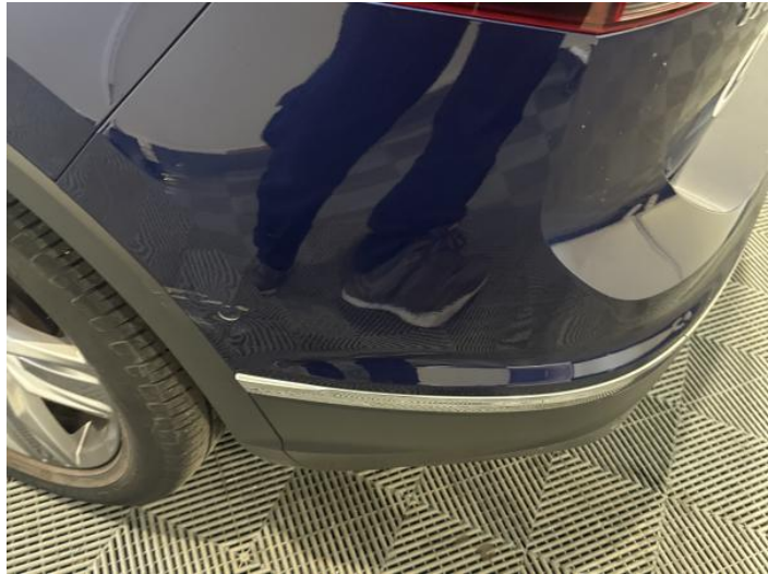
10: Bumper Rear Scratched Over 100mm Thru Paint
