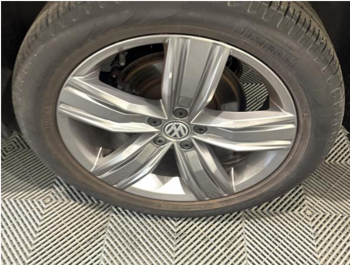
9: Wheel nsr Scratched Over 50mm
