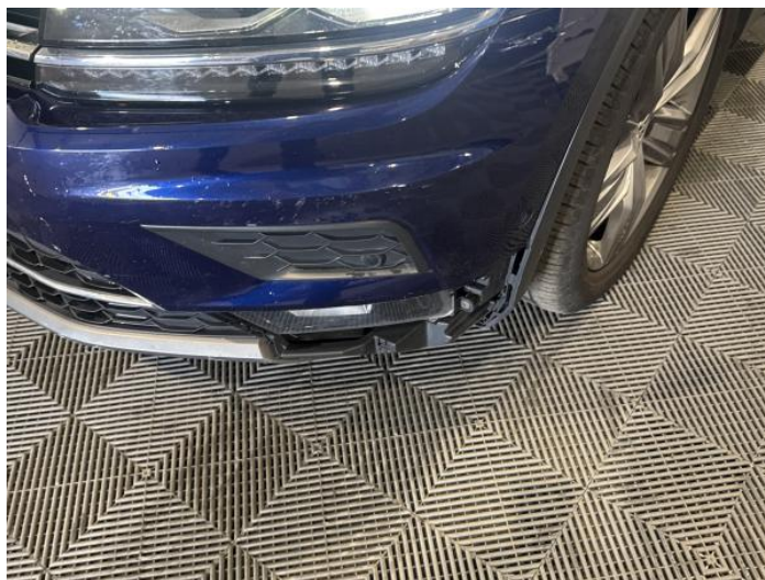
2: Bumper Front Scratched Over 100mm Thru Paint
