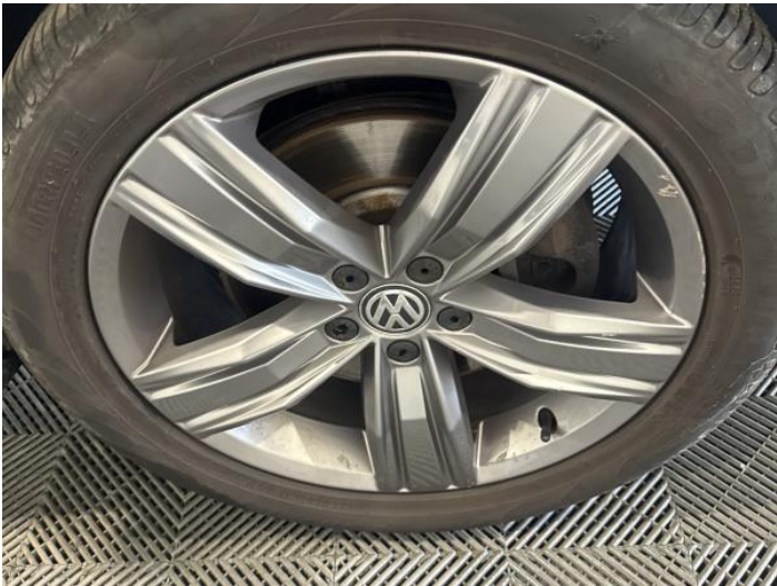
17: Wheel osf Scratched Over 50mm
