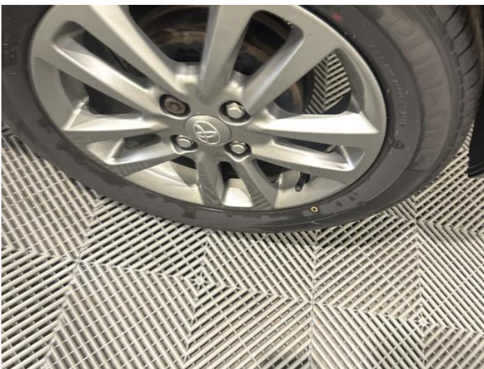
7: Wheel nsr Scratched Up To 50mm
