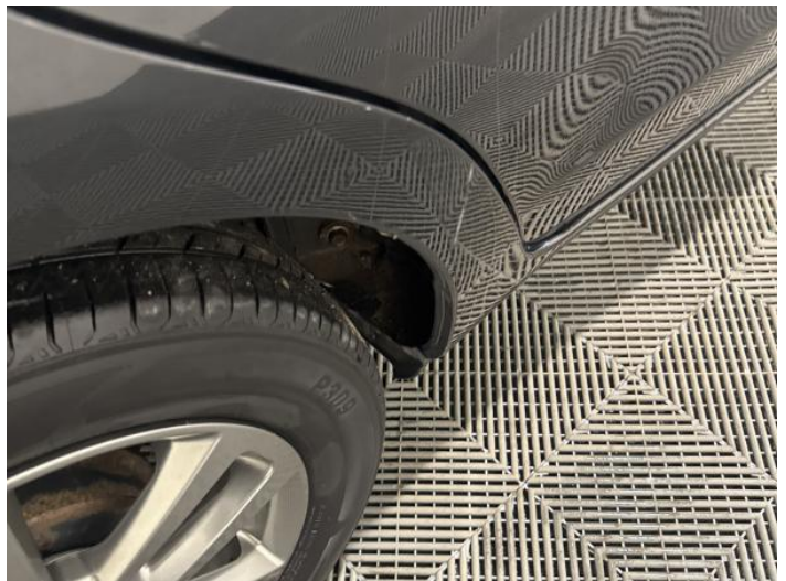
10: Qtr Panel osr Dented With Paint Damage
