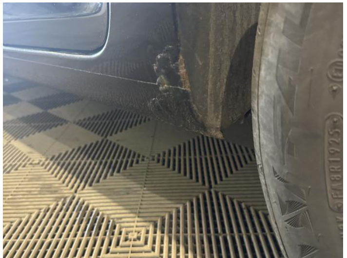
12: Sill ns Rusted Over 5mm
