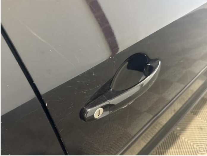
21: Door osf Scratched Over 25mm Thru Paint
