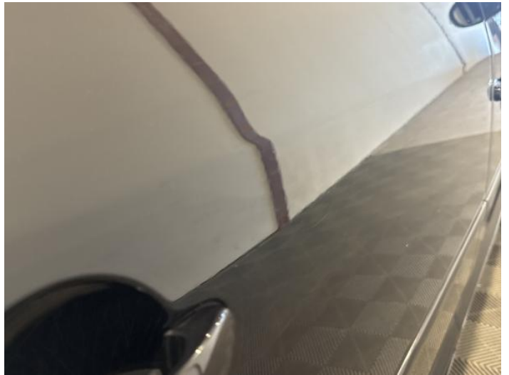
18: Door osr Dented Between 10mm + 30mm
