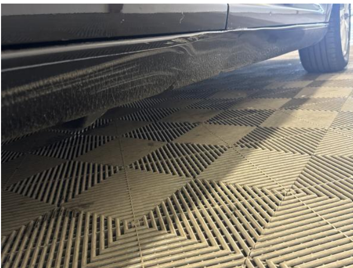
19: Sill os Dented With Paint Damage
