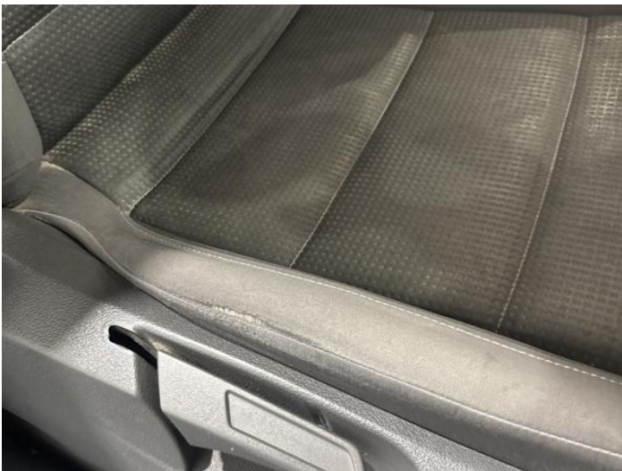
1: Seat Back Cover osf Scuffed Over 25mm
