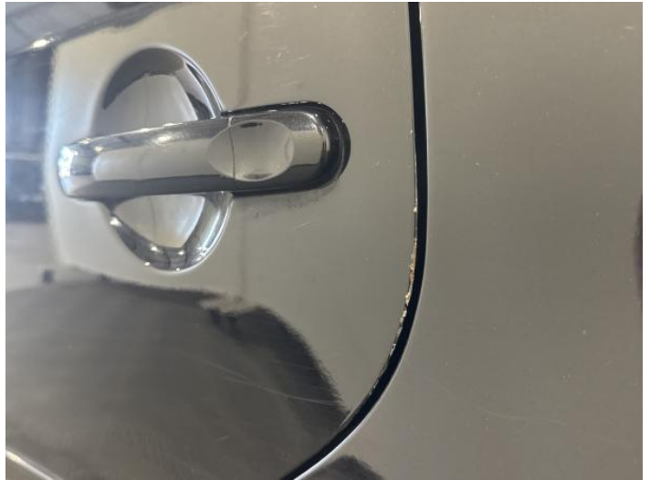
10: Door nsr Scratched Rusted
