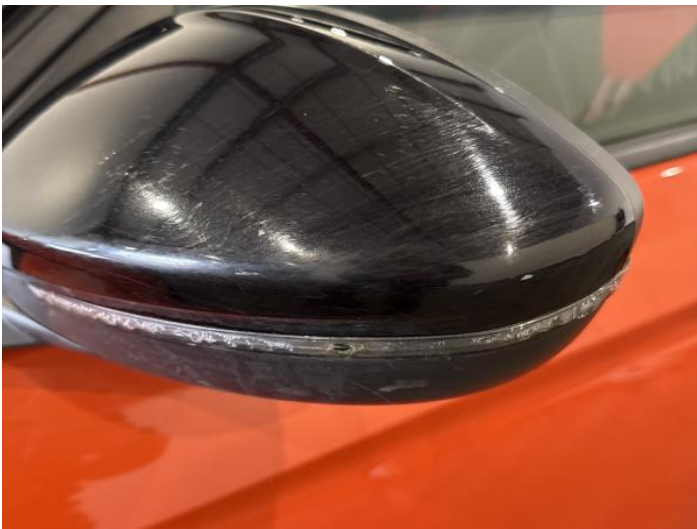
5: Flasher Side Repeater ns Broken Replace
