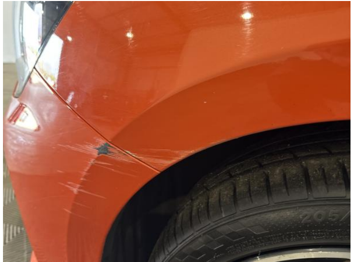
4: Wing nsf Scratched Over 25mm Thru Paint
