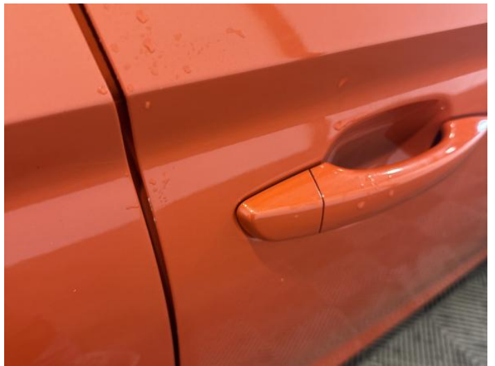
12: Door osf Chipped Edge Chip
