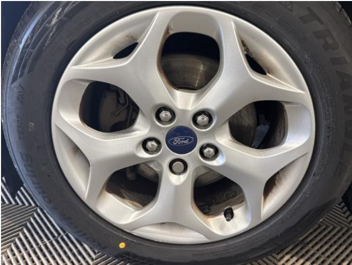
3: Wheel nsf Scratched Over 50mm
