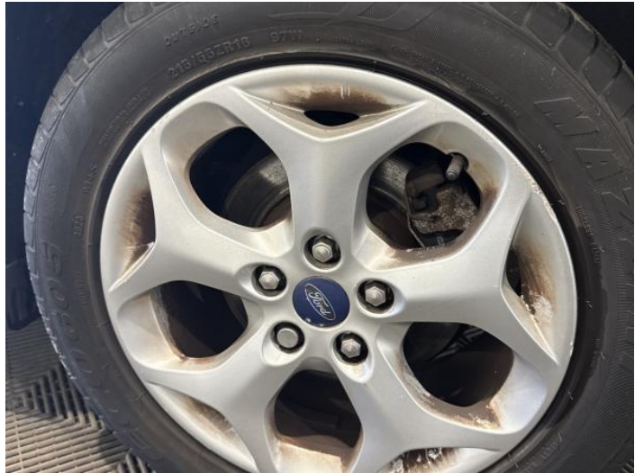
10: Wheel nsr Scratched Over 50mm
