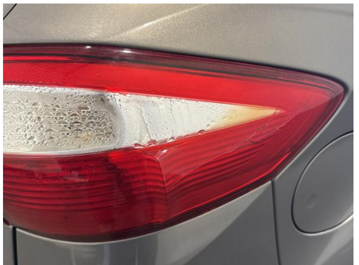
14: Lamp osr Broken Replace
