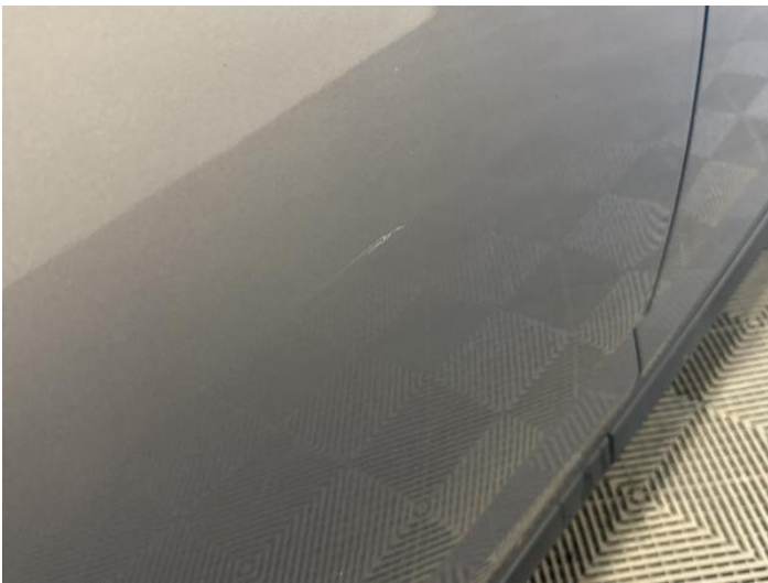
17: Door osr Scratched Over 25mm Thru Paint
