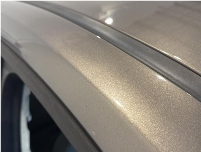
21: A Post os Dented Over 30mm
