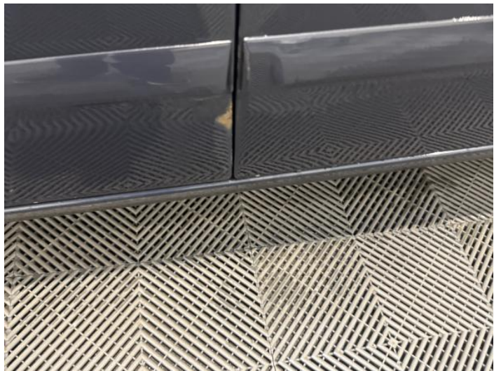
6: Door nsf Rusted Over 5mm
