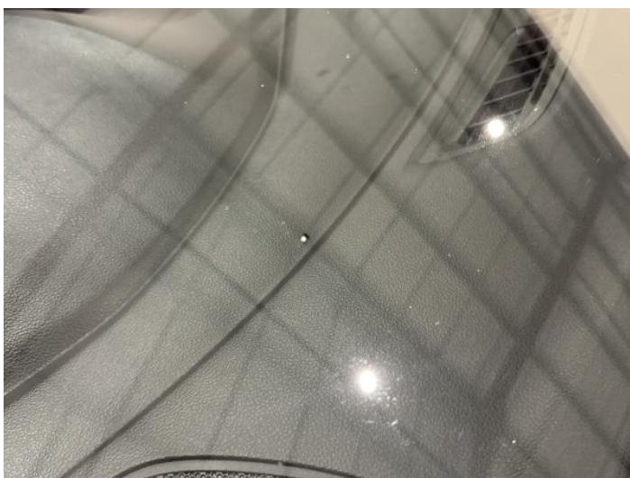
19: Screen Front Chipped UpTo 10mm
