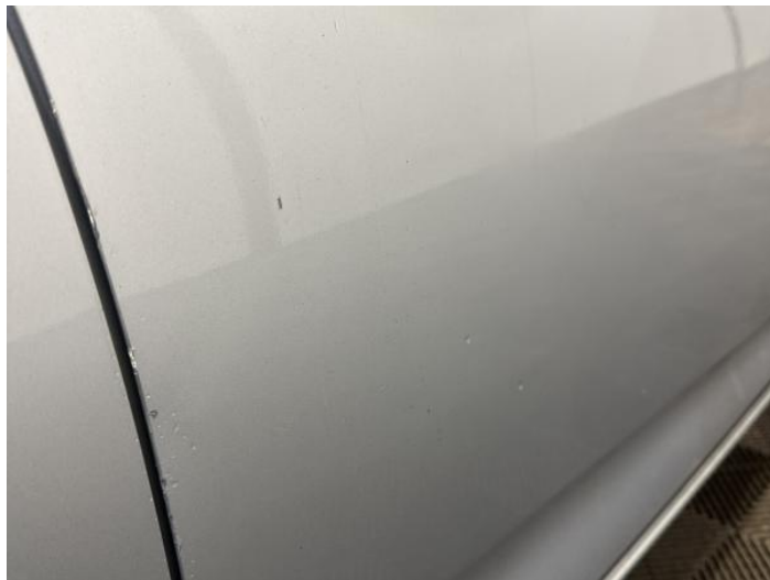
16: Door osf Scratched Over 25mm Thru Paint
