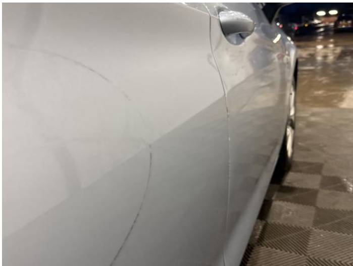
15: Door osr Dented Over 2 UpTo 10mm
