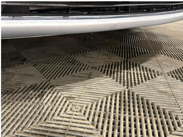
21: Bumper Front Moulding Missing Replace
