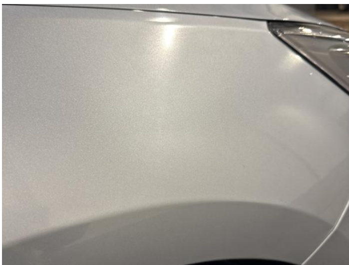
17: Wing osf Poor Previous Repair Poor Paint
