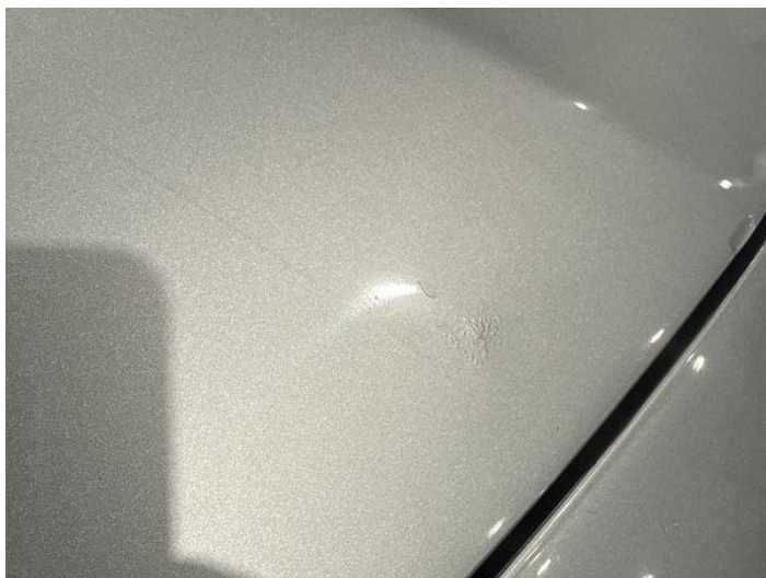
1: Bonnet Poor Previous Repair Rippled Up To 30%
