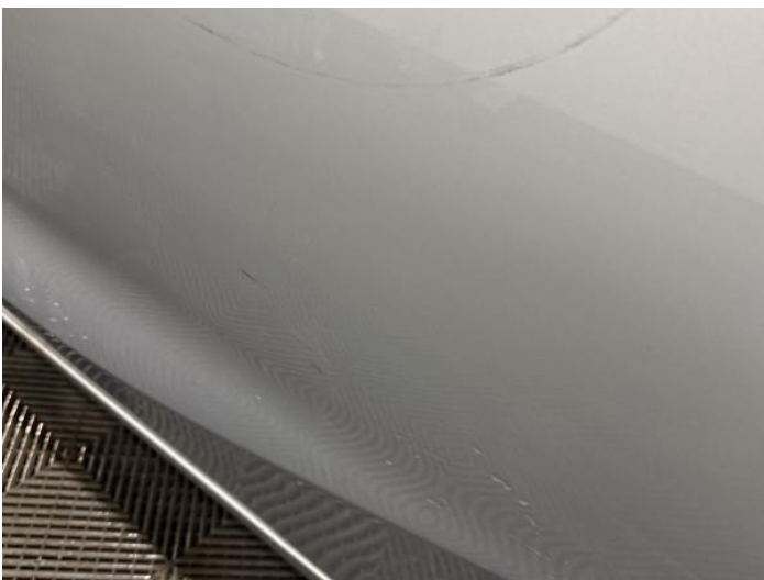
7: Door nsr Poor Previous Repair Rippled UpTo 30%
