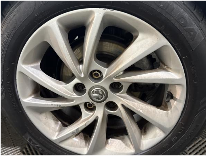
9: Wheel nsr Scratched Over 50mm
