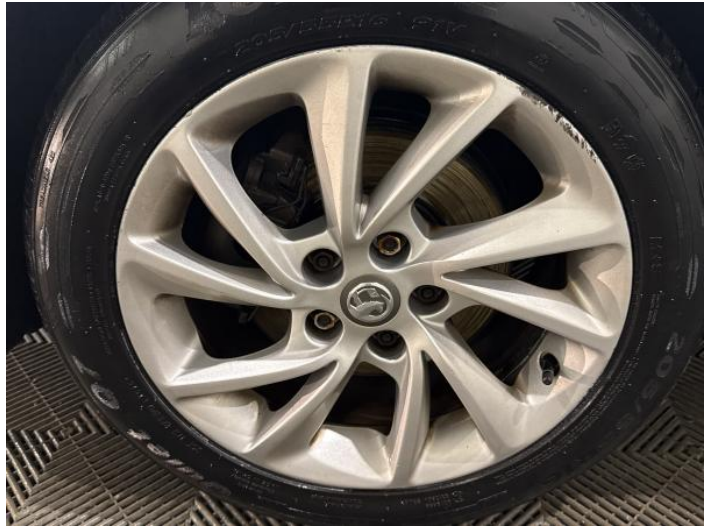
4: Wheel nsf Scratched Over 50mm
