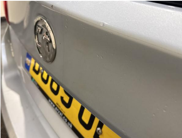
11: Tailgate Poor Previous Repair Rippled UpTo 30%
