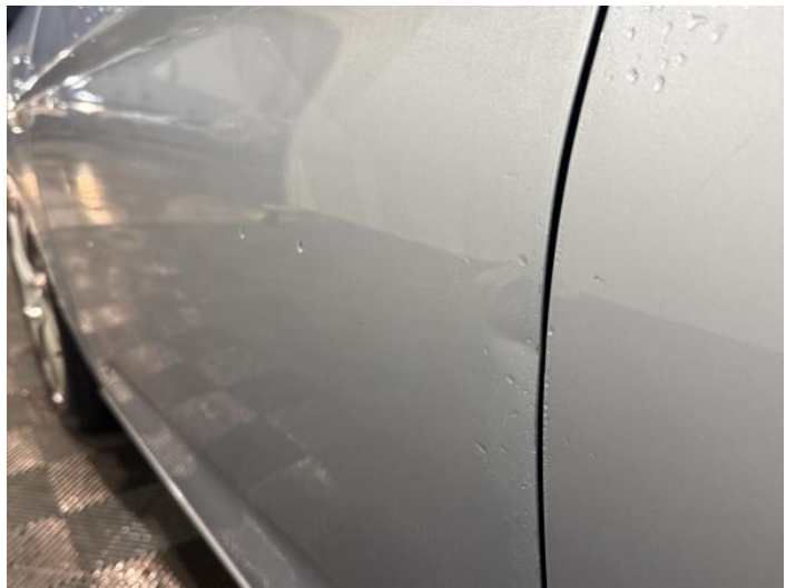
6: Door nsf Poor Previous Repair Rippled UpTo 30%
