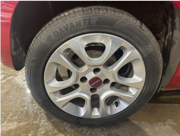
5: Wheel osr Scratched Over 50mm
