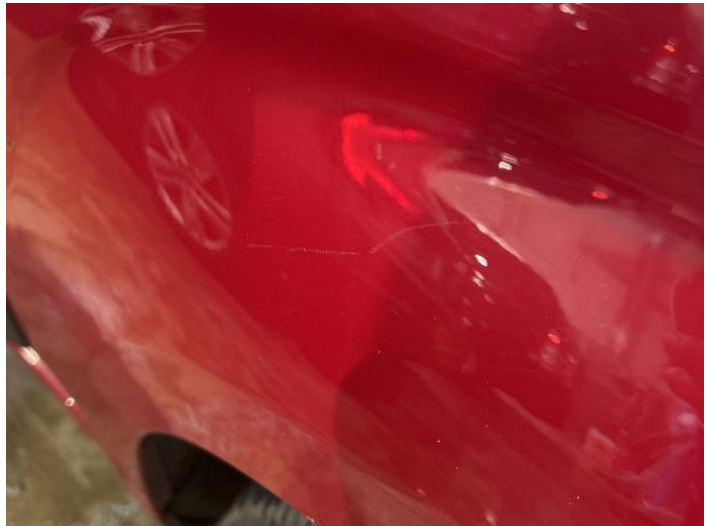
2: Wing osf Scratched Over 25mm Not Thru Paint
