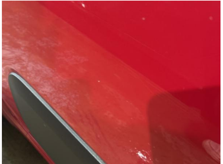
4: Door osr Chipped 1 To 5
