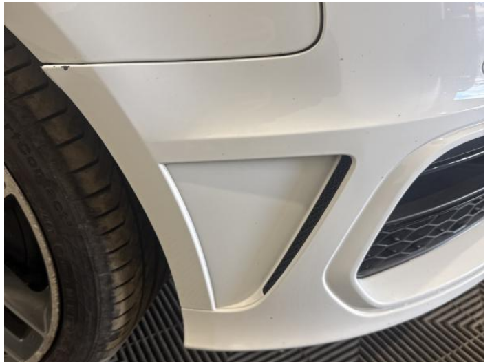
2: Bumper Front Scratched 25 to 100mm Thru Paint
