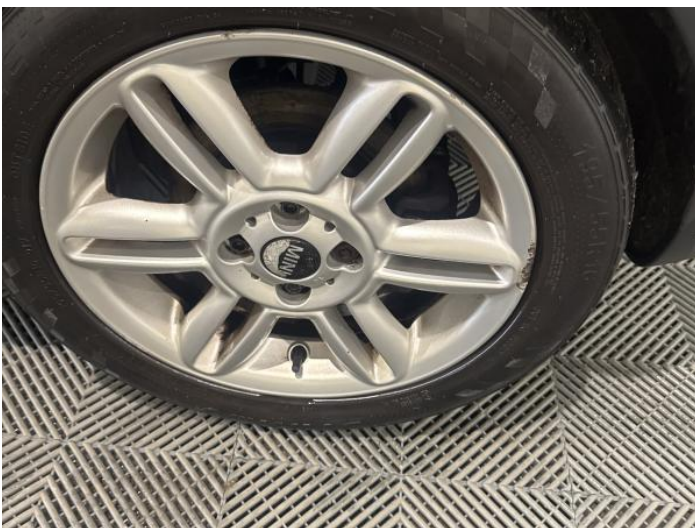
7: Wheel nsr Scratched Over 50mm
