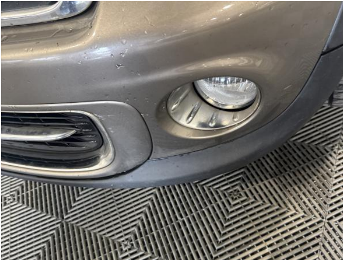
3: Bumper Front Scratched Over 100mm Thru Paint
