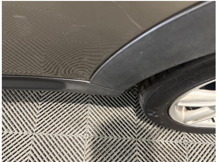
6: Qtr Panel nsr Dented With Paint Damage
