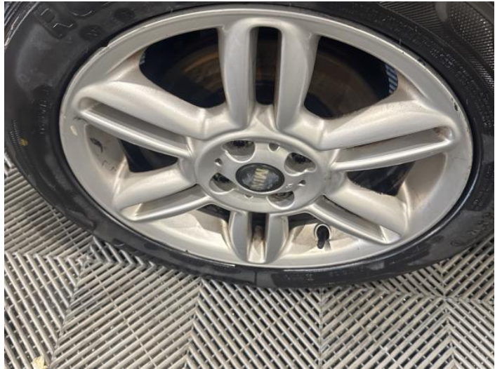
4: Wheel nsf Scratched Over 50mm
