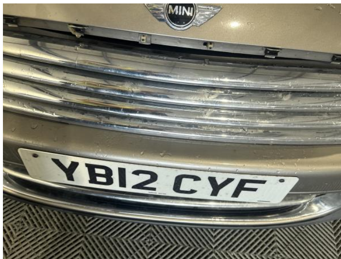
2: Bumper Front Grill Broken Replace
