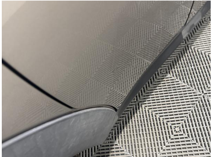
10: Door osr Dented Over 2 UpTo 10mm
