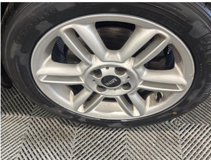
13: Wheel osf Scratched Over 50mm
