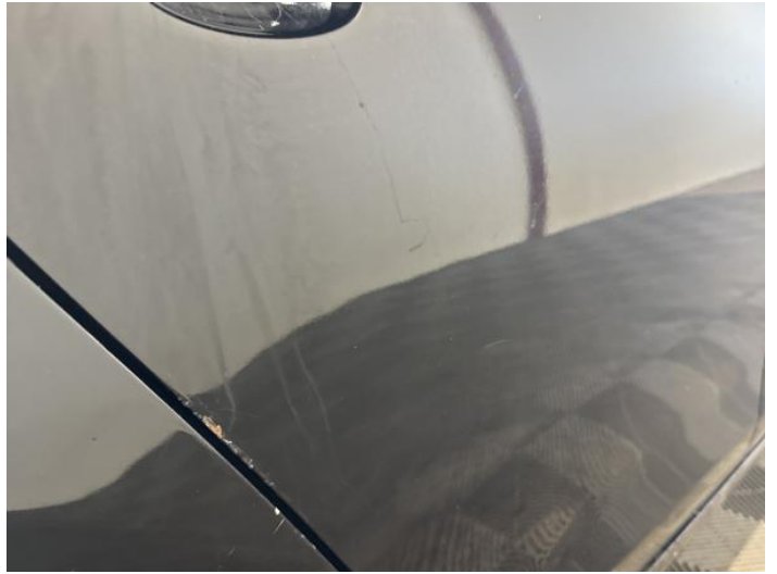
16: Door osr Scratched Rusted
