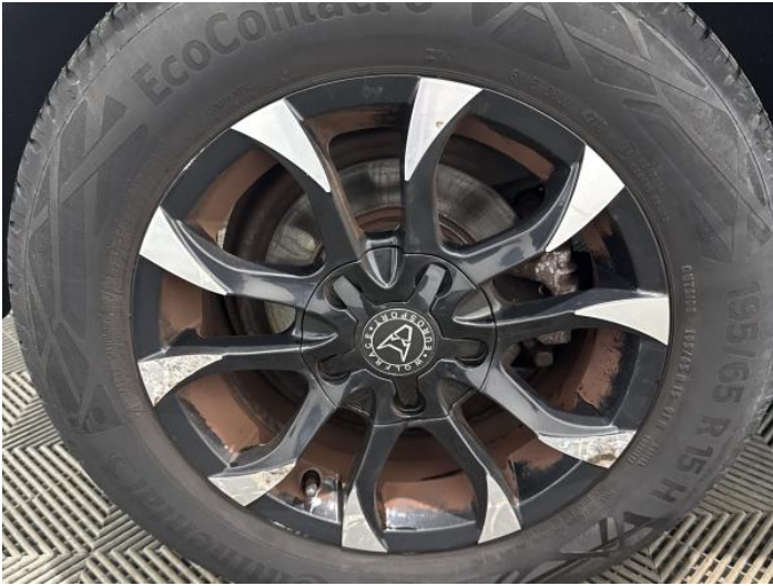
15: Wheel osr Scratched Over 50mm
