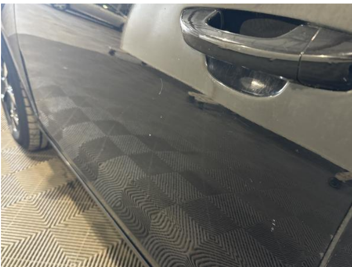
7: Door nsf Scratched Over 25mm Thru Paint
