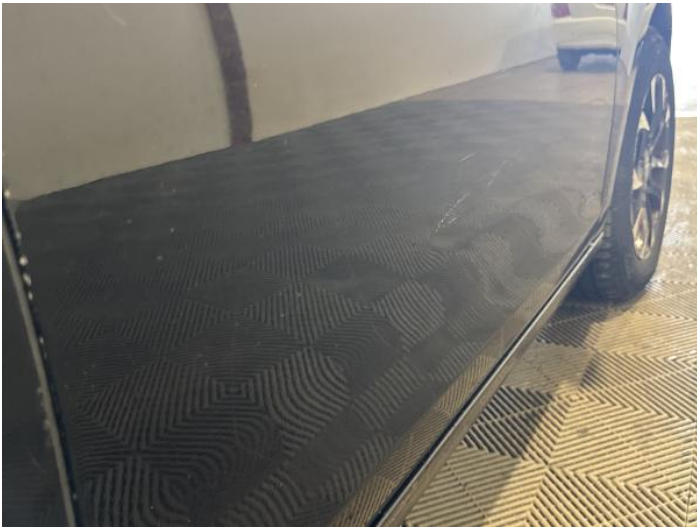
17: Door osf Dented With Paint Damage
