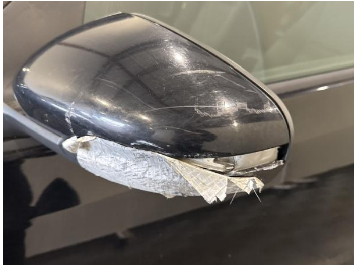
4: Door Mirror Assy nsf Broken Replace
