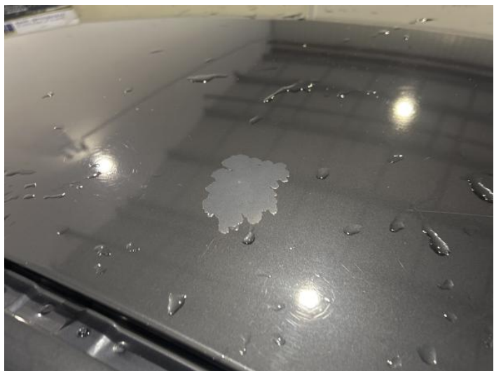
14: Roof Poor Previous Repair Paint Flake
