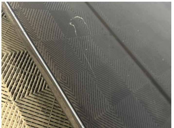
8: Door nsr Scratched Over 25mm Thru Paint
