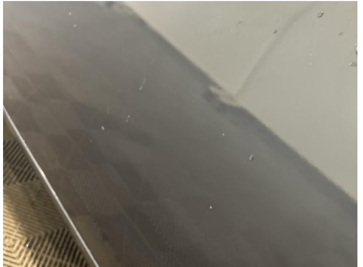
10: Door nsf Poor Previous Repair Poor Paint
