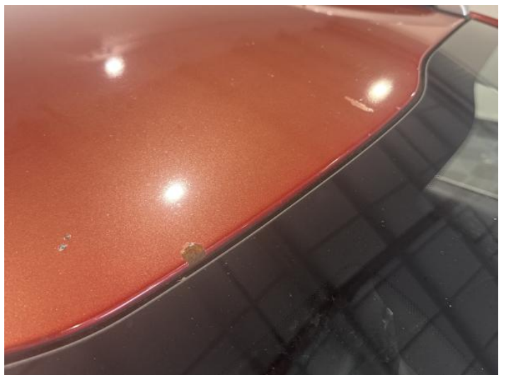
20: Roof Poor Previous Repair Paint Flake
