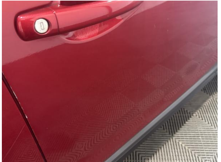
16: Door osf Scratched Over 25mm Thru Paint
