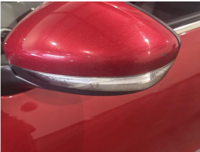
5: Flasher Side Repeater ns Broken Replace
