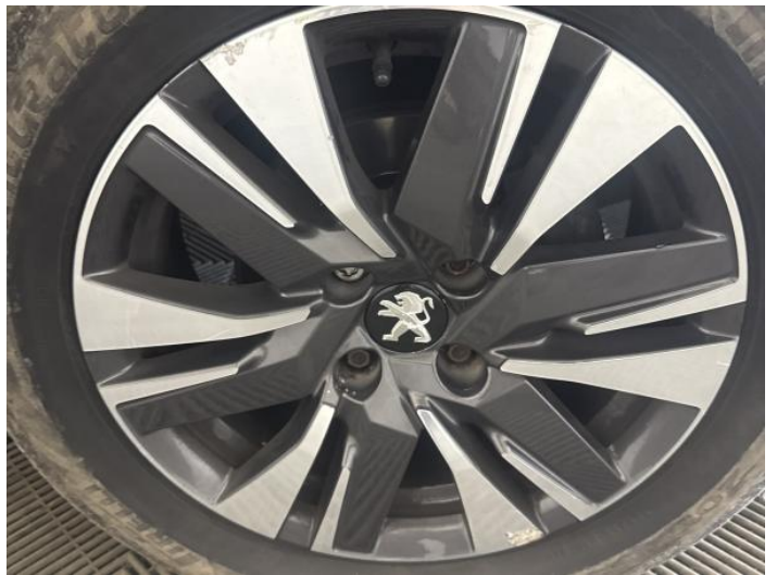
18: Wheel osf Scratched Over 50mm
