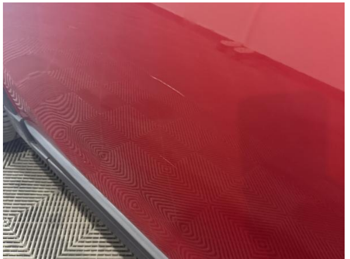
6: Door nsf Scratched Over 25mm Thru Paint
