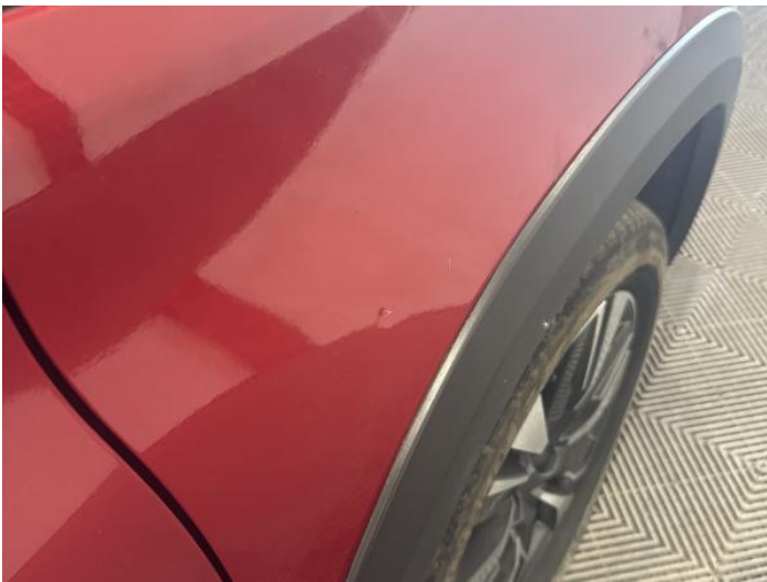
17: Wing osf Dented Between 10mm + 30mm
