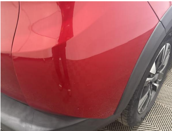
11: Bumper Rear Moulding Scratched (Painted) Over 25mm Thru Paint
