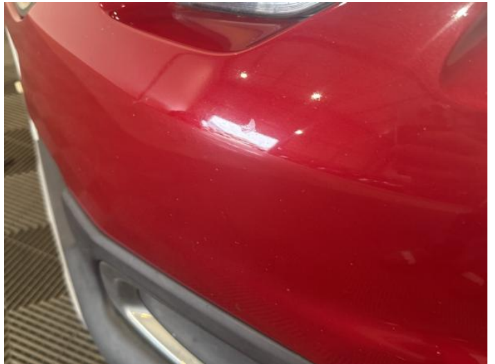
2: Bumper Front Poor Previous Repair Paint Flake
