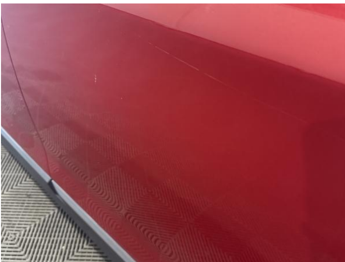
7: Door nsr Scratched Over 25mm Thru Paint
