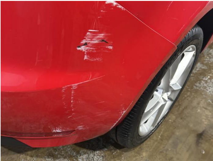
5: Bumper Rear Scratched Over 100mm Thru Paint
