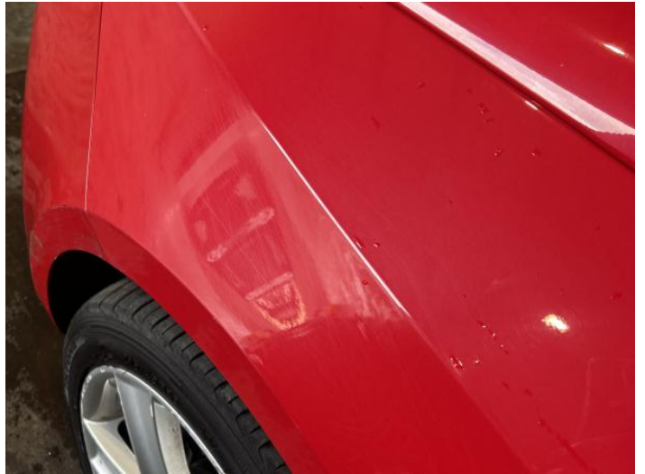
10: Wing nsf Scratched Over 25mm Not Thru Paint
