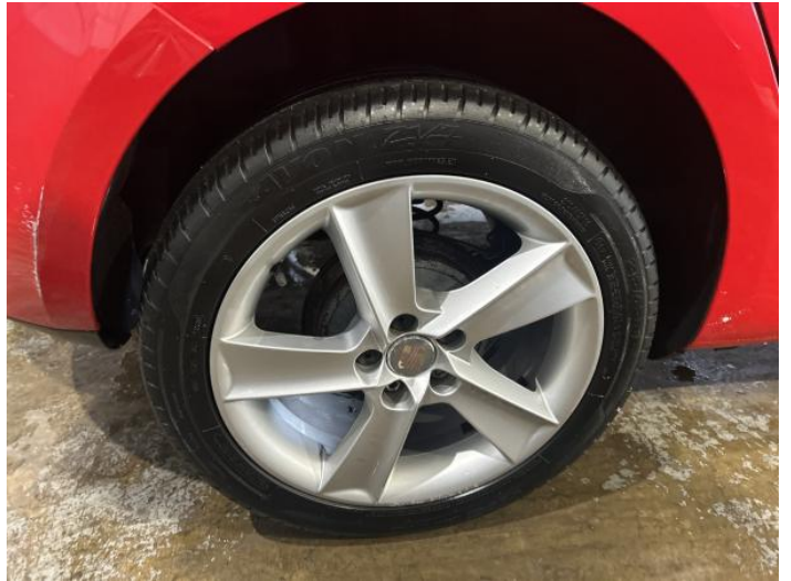
4: Wheel osr Scratched Over 50mm
