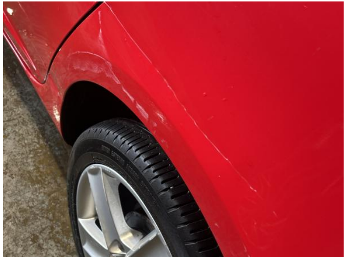
6: Qtr Panel nsr Dented With Paint Damage
