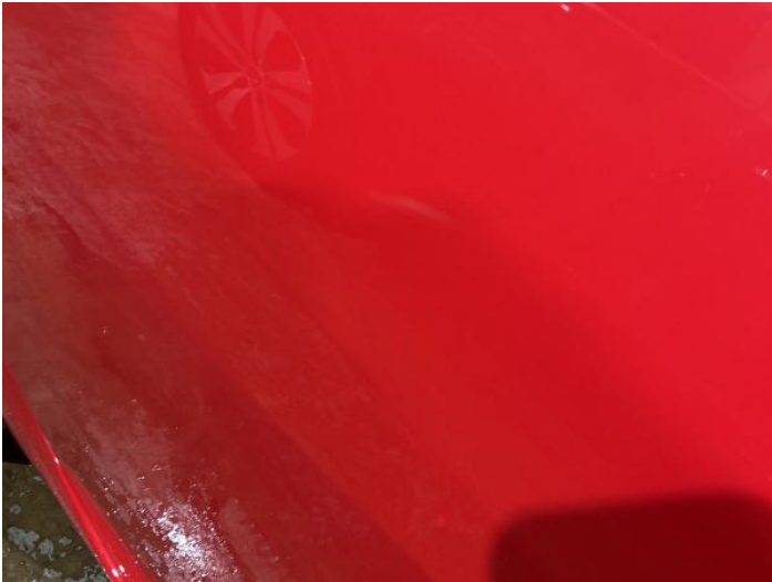
3: Door osr Scratched UpTo 25mm Not Thru Paint
