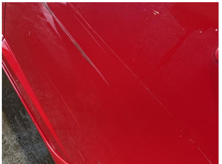
8: Door nsr Scratched Over 25mm Thru Paint
