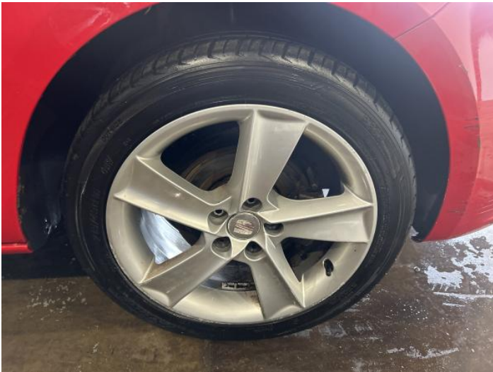
1: Wheel osf Scratched Over 50mm
