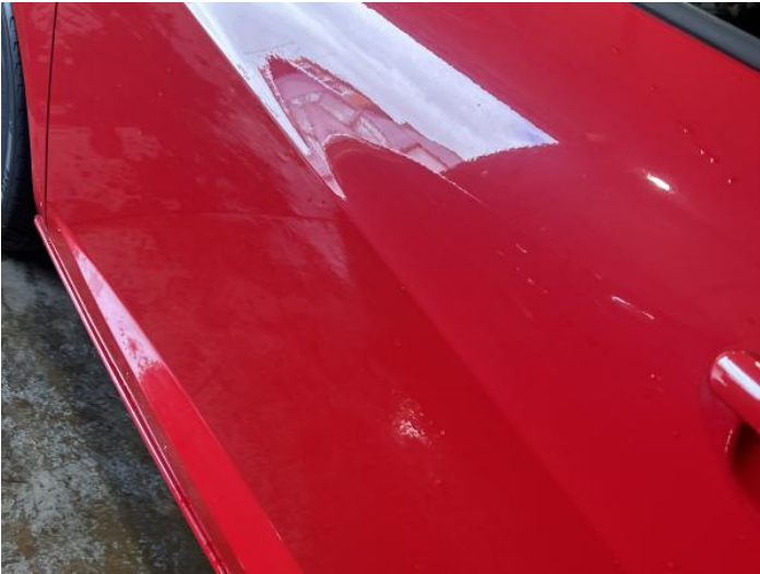
9: Door nsf Scratched Over 25mm Not Thru Paint
