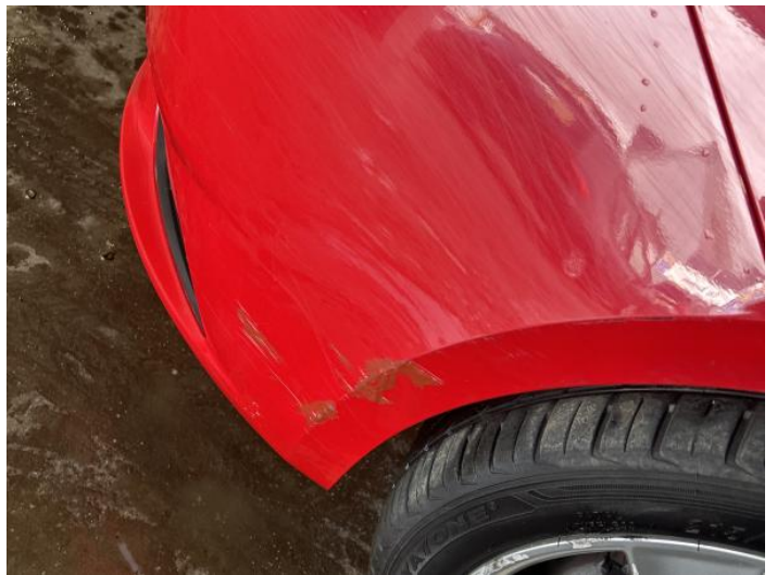
12: Bumper Front Scratched Over 100mm Thru Paint
