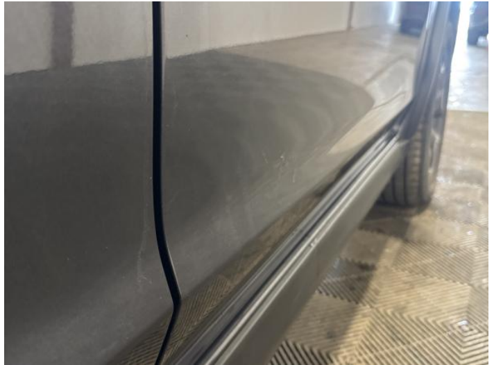
10: Door osf Dented Over 30mm
