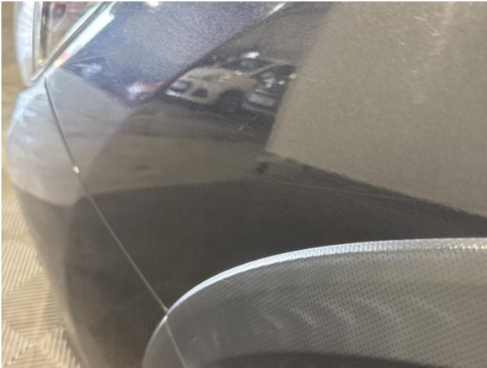
3: Wing nsf Scratched UpTo 25mm Thru Paint
