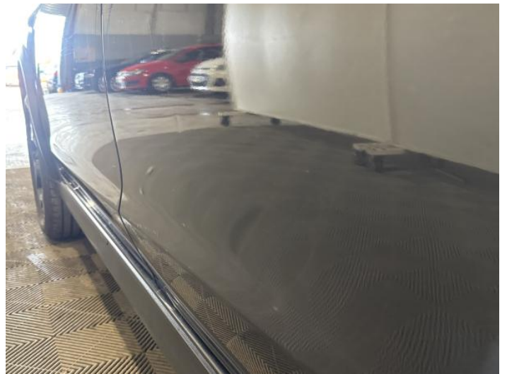
6: Door nsr Dented Between 10mm + 30mm
