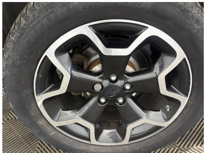
8: Wheel osr Scratched Over 50mm
