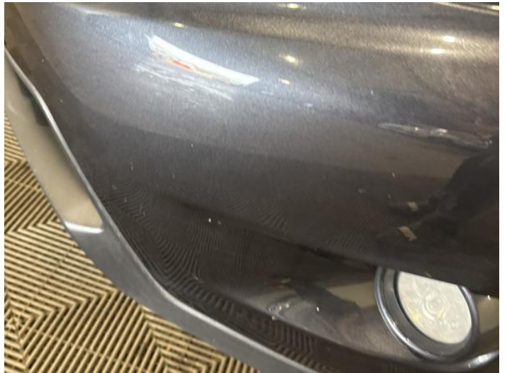
2: Bumper Front Chipped Multiple Chips
