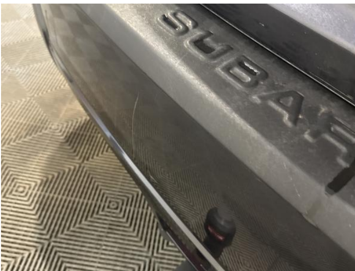
7: Bumper Rear Scratched 25 to 100mm Thru Paint
