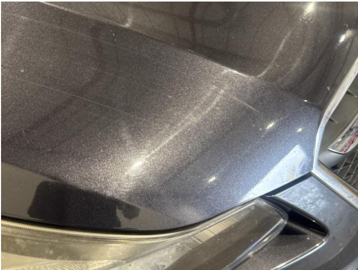
1: Bonnet Scratched Over 25mm Thru Paint
