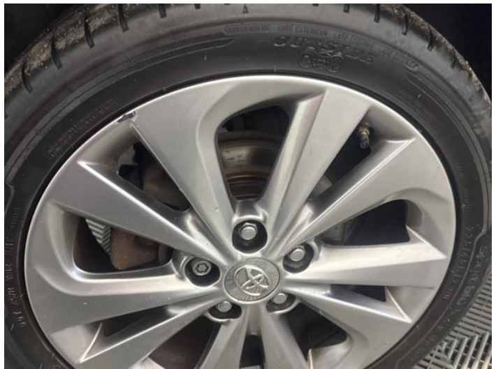
12: Wheel osr Scratched Up To 50mm
