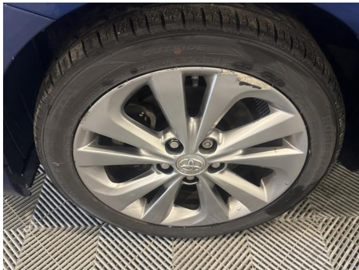
4: Wheel nsf Scratched Over 50mm
