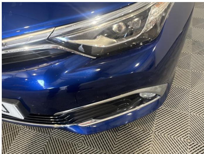
2: Bumper Front Scratched 25 to 100mm Thru Paint
