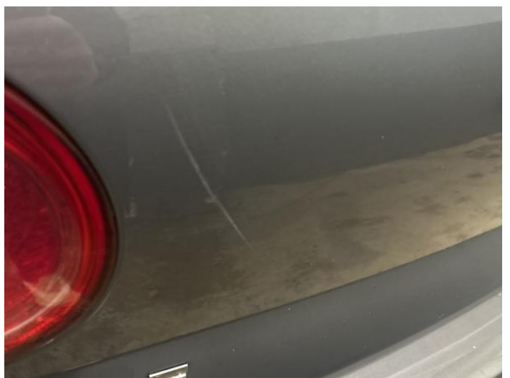
8: Tailgate Scratched Over 25mm Not Thru Paint
