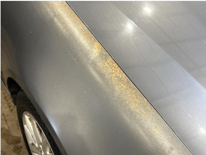
1: Wing of Poor Previous Repair Poor Paint
