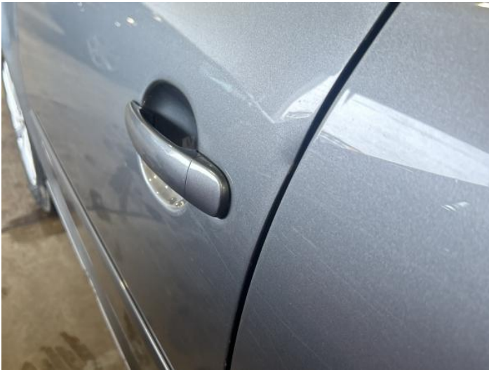
11: Door nsf Dented Over 30mm
