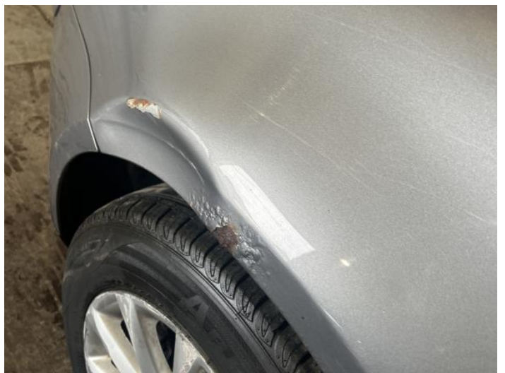
14: Wing nsf Dented With Paint Damage
