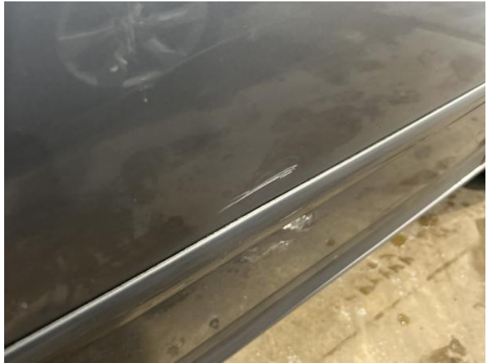
4: Door osf Dented With Paint Damage
