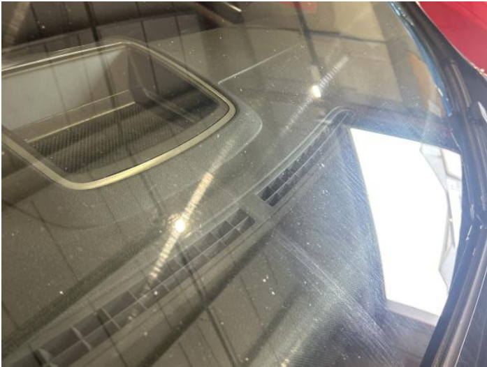
21: Screen Front Chipped UpTo 10mm
