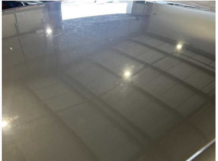
22: Roof Scratched Over 25mm Not Thru Paint
