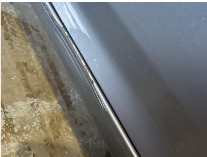
13: Sill ns Dented With Paint Damage
