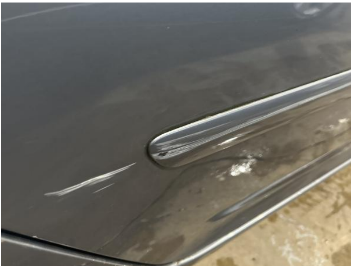
5: Door osr Scratched Over 25mm Thru Paint
