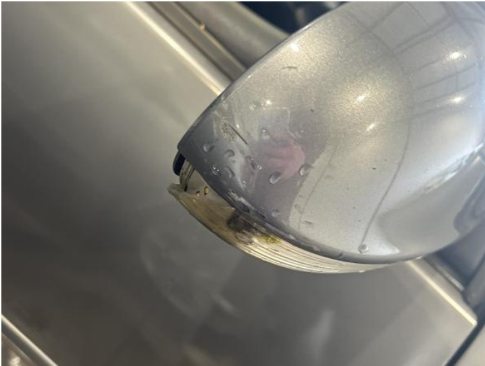
3: Door Mirror Assy osf Broken Replace
