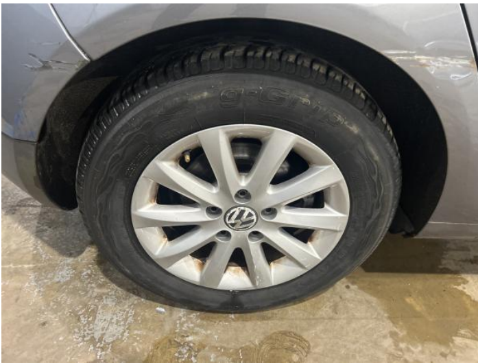
23: Wheel osr Scratched Over 50mm
