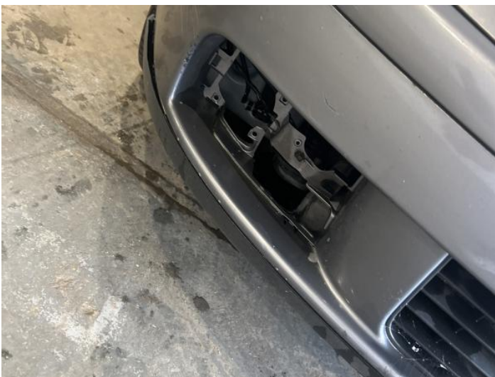
19: Fog Lamp Surround os Missing Replace
