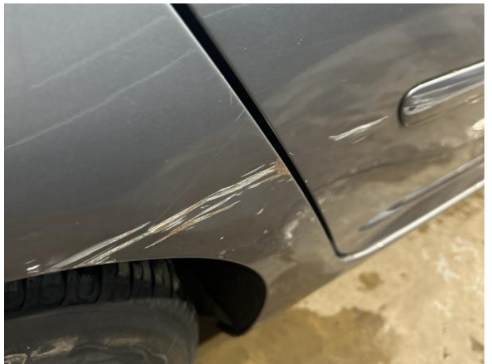
6: Qtr Panel osr Dented With Paint Damage
