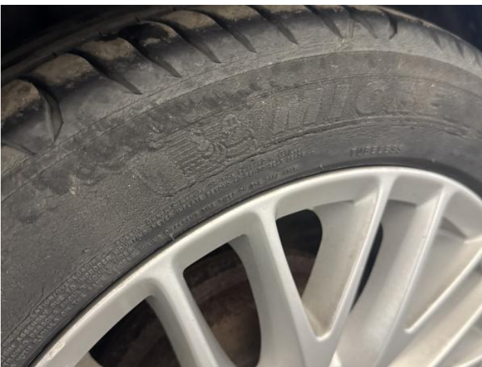
25: Tyre osr Damaged Replace
