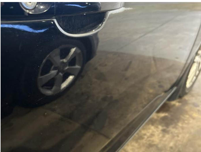
7: Door osf Scratched Over 25mm Not Thru Paint
