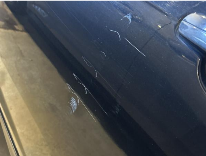
15: Door nsr Scratched Over 25mm Thru Paint
