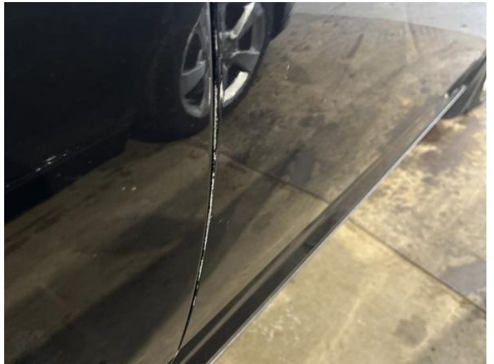
6: Door osf Chipped Edge Chip
