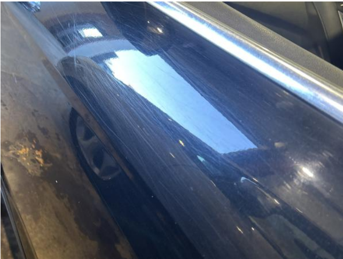
17: Door nsf Scratched Over 25mm Not Thru Paint
