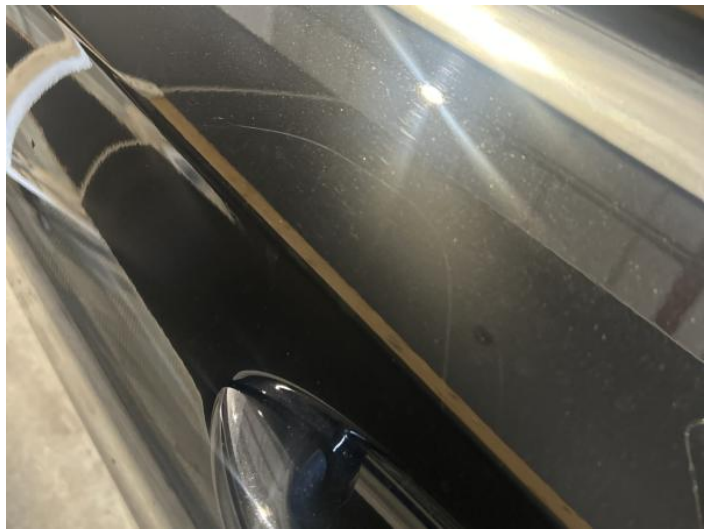
6: Door nsr Scratched Over 25mm Not Thru Paint
