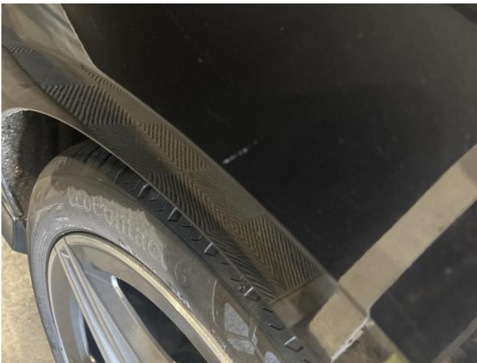
5: Qtr Panel nsr Scratched UpTo 25mm Not Thru Paint
