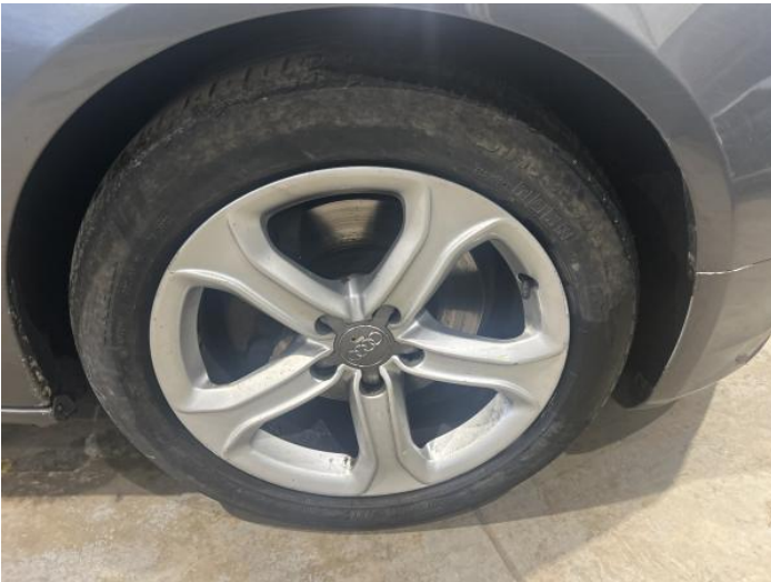
1: Wheel osf Scratched Over 50mm
