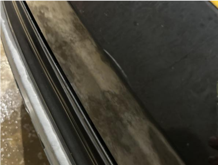
9: Tailgate Scratched UpTo 25mm Not Thru Paint
