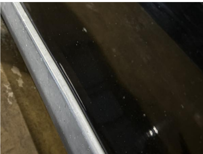
13: Door nsf Scratched Over 25mm Thru Paint
