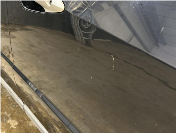
3: Door osf Dented With Paint Damage
