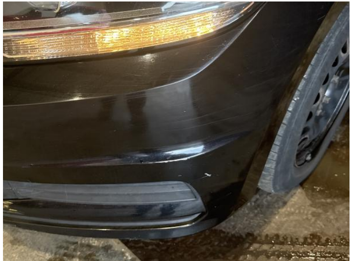
2: Bumper Front Scratched Over 100mm Thru Paint
