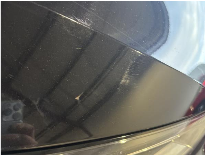
1: Bonnet Chipped Multiple Chips
