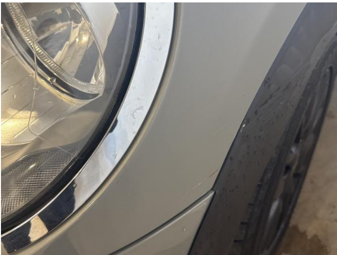
1: Bonnet Scratched Over 25mm Thru Paint
