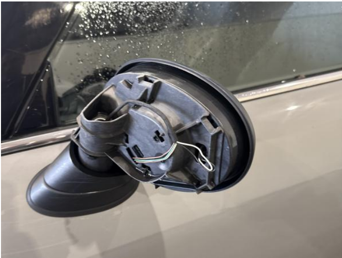
5: Door Mirror Assy nsf Broken Replace
