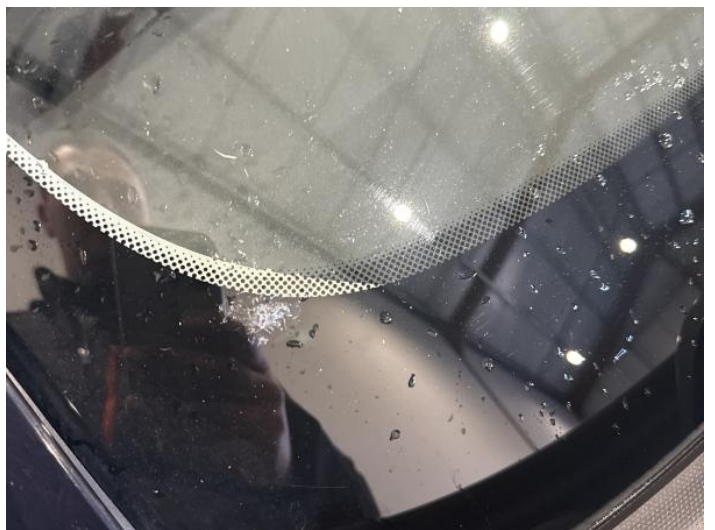
14: Screen Front Cracked Replace
