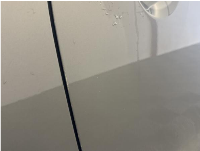
11: Door osf Chipped Edge Chip
