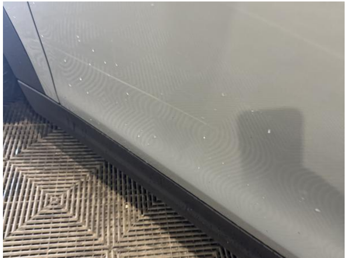
6: Door nsf Scratched Over 25mm Thru Paint
