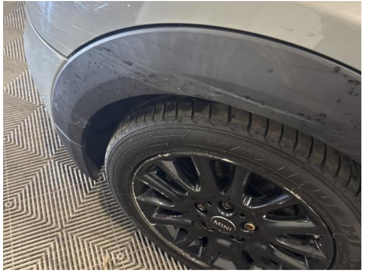
4: Wing Front Arch Extension ns Scuffed (Unpainted) Over 100mm
