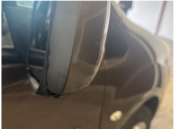
18: Door Mirror Assy nsf Broken Replace
