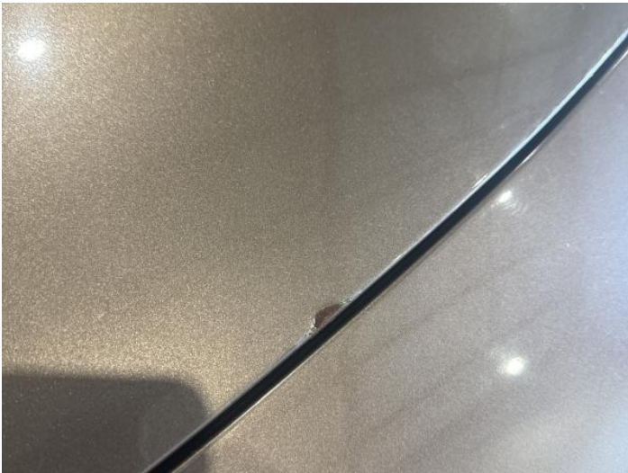
1: Bonnet Scratched Rusted
