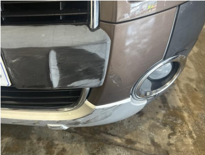
3: Bumper Front Moulding Scuffed (Unpainted) Over 100mm
