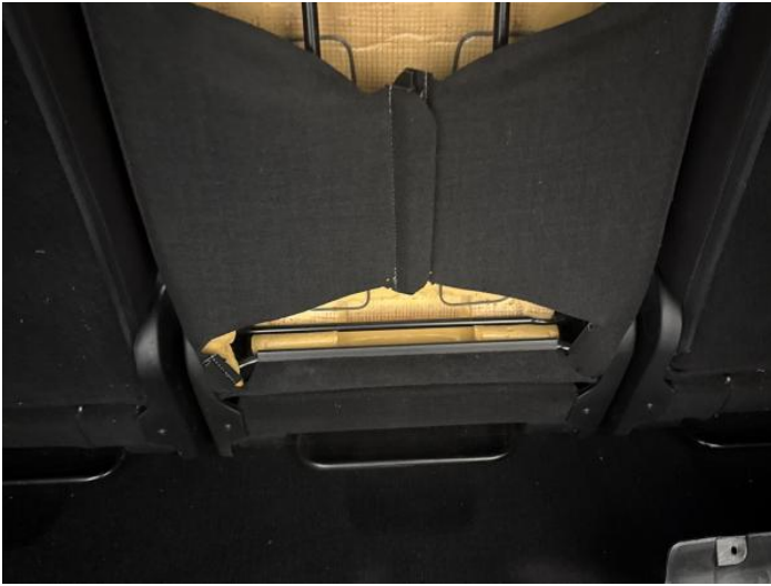
21: Seat Back Cover nsr Scuffed Over 25mm
