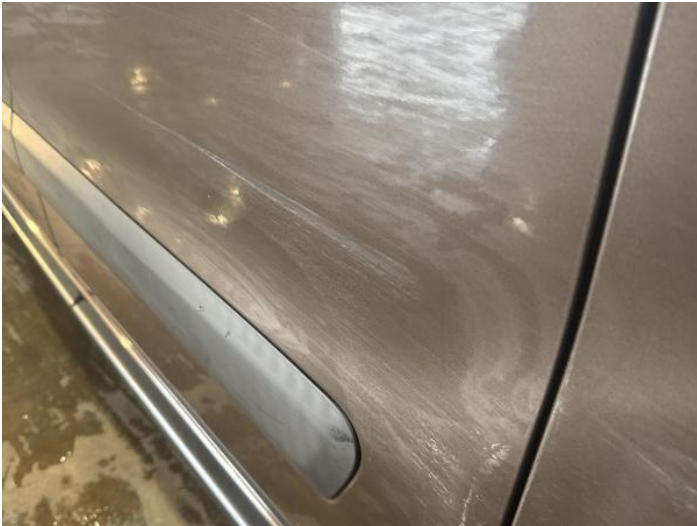
9: Door nsr Scratched Over 25mm Thru Paint
