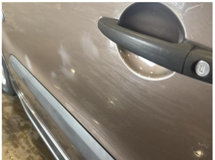
8: Door nsf Scratched Over 25mm Thru Paint
