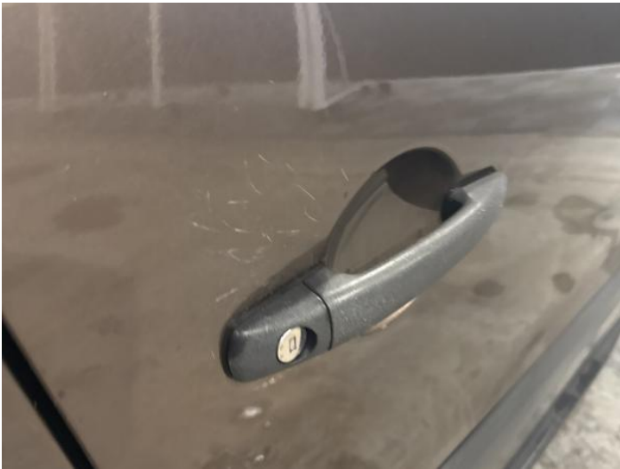
17: Door osf Scratched Over 25mm Thru Paint
