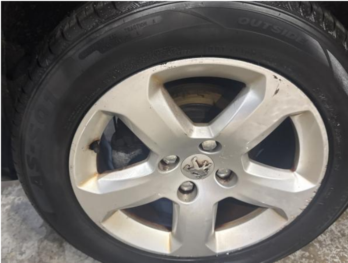
15: Wheel osr Scratched Over 50mm
