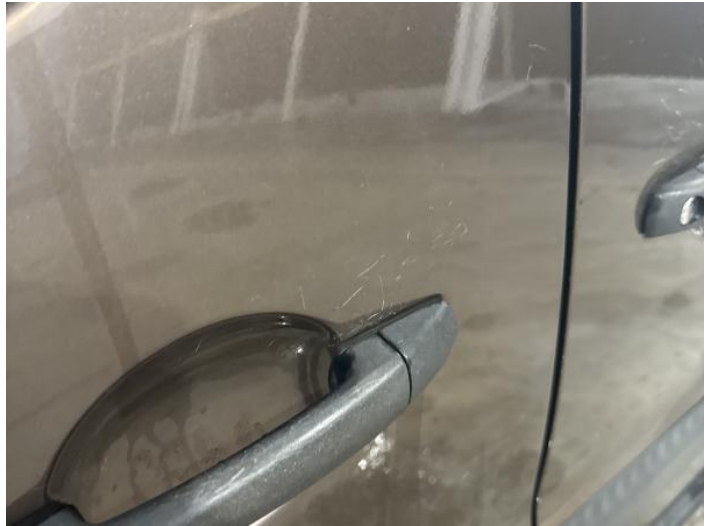
16: Door osr Scratched Over 25mm Thru Paint
