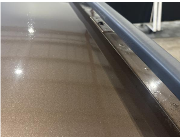
13: Roof Dented Between 10mm + 30mm
