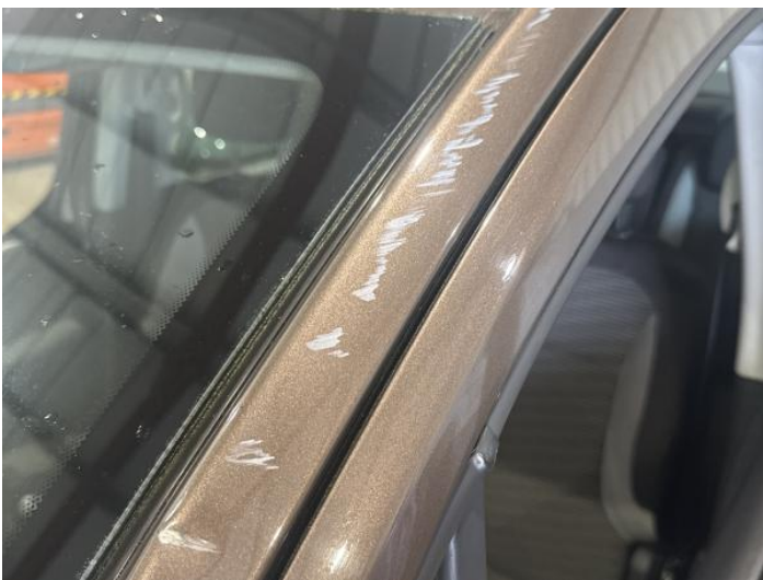
7: A Post ns Dented With Paint Damage
