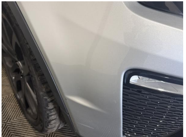
2: Bumper Front Scratched 25 to 100mm Thru Paint
