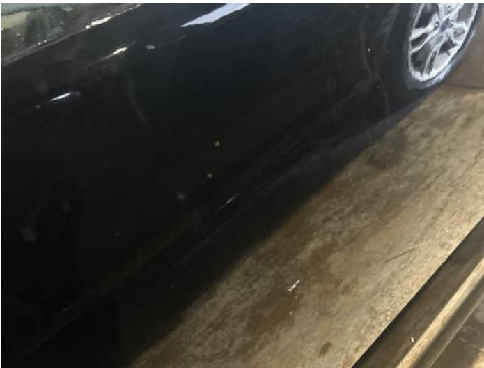
1: Door osf Chipped 1 To 5
