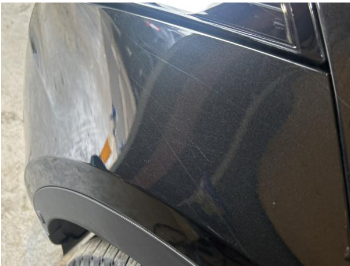
5: Bumper Front Scratched Over 25mm Not Thru Paint
