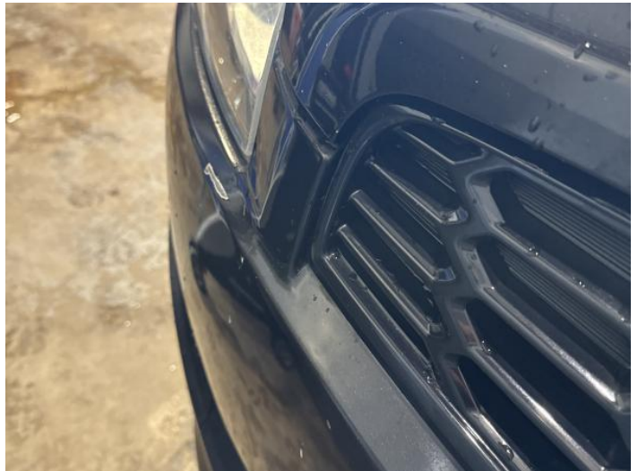
2: Bumper Front Scratched 25 to 100mm Thru Paint
