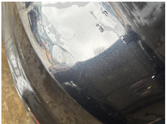
8: Bumper Rear Poor Previous Repair Paint Flake
