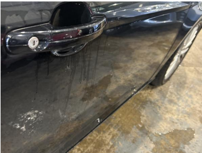
5: Door osf Scratched Over 25mm Not Thru Paint
