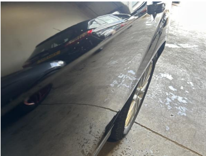
23: Door nsr Dented Over 2 UpTo 10mm
