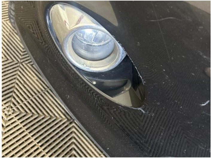
28: Bumper Front Scratched 25 to 100mm Thru Paint
