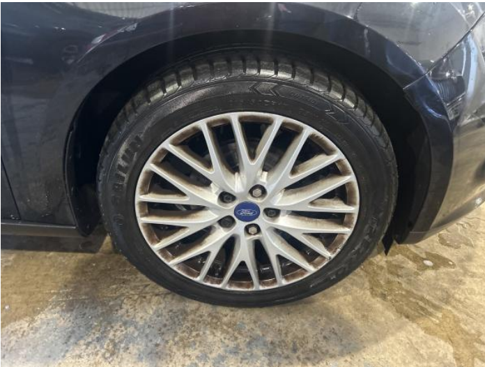
1: Wheel of Scratched Over 50mm
