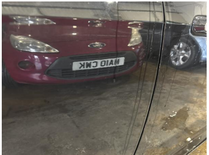
6: Door osr Scratched Over 25mm Not Thru Paint
