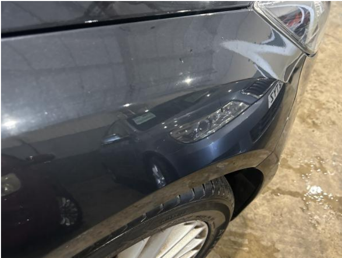
3: Wing osf Scratched Over 25mm Not Thru Paint
