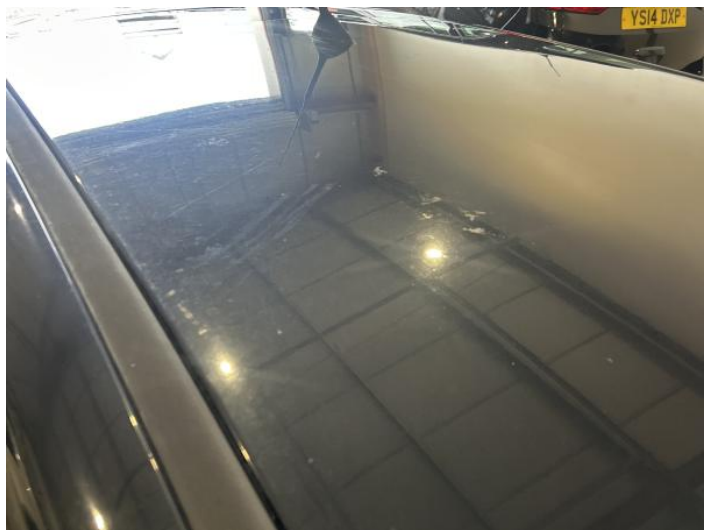
26: Roof Scratched Over 25mm Not Thru Paint
