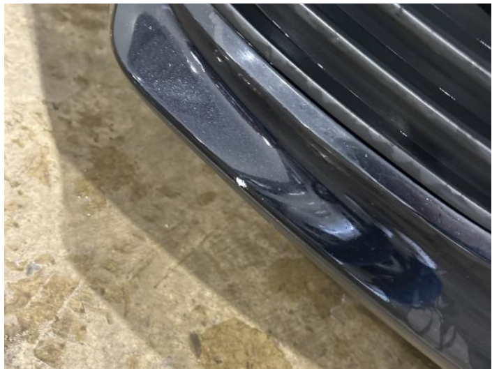
18: Bumper Front Chipped Multiple Chips
