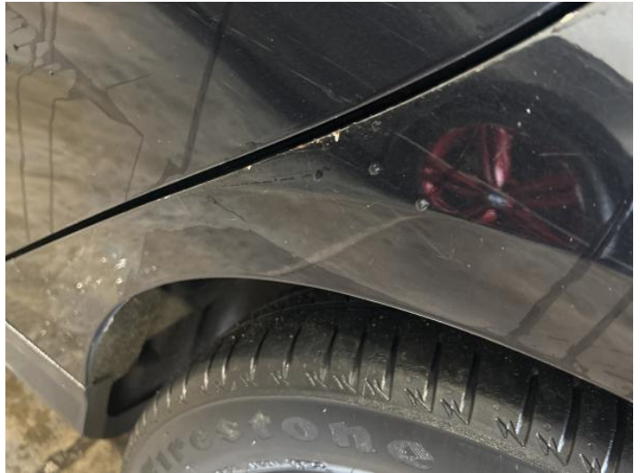
10: Qtr Panel nsr Chipped 1 To 5
