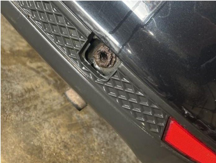
9: Rear TowEye Cvr Missing Replace
