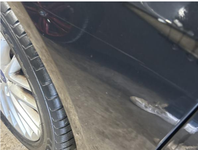
17: Wing nsf Scratched Over 25mm Not Thru Paint
