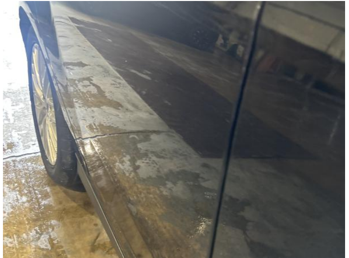
22: Door osr Dented Between 10mm + 30mm
