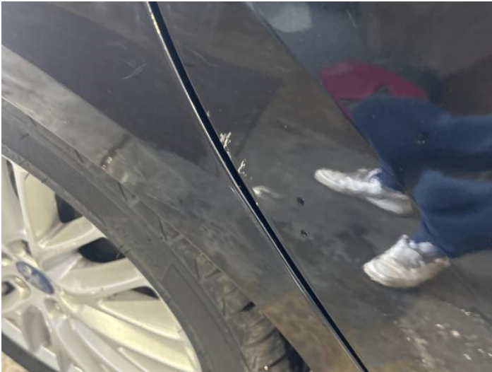
21: Door osr Chipped 1 To 5
