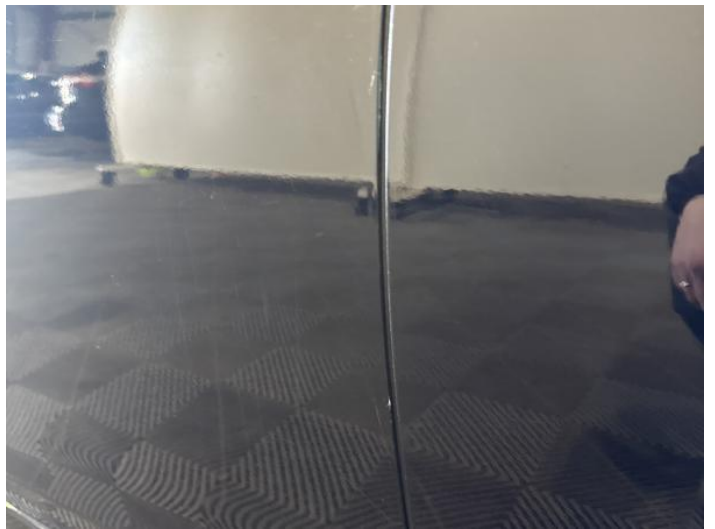
6: Door nsf Scratched Up To 25mm Thru Paint
