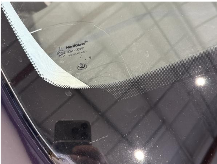
5: Screen Front Cracked Replace
