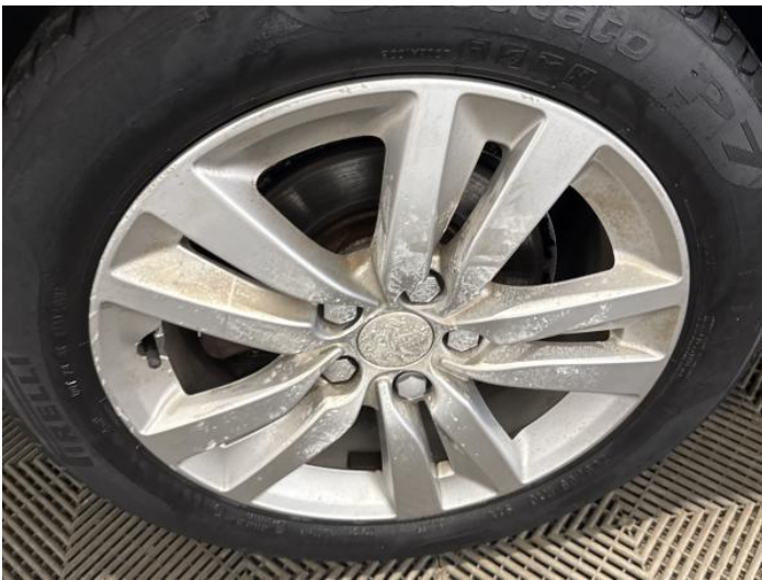
11: Wheel osr Scratched Over 50mm
