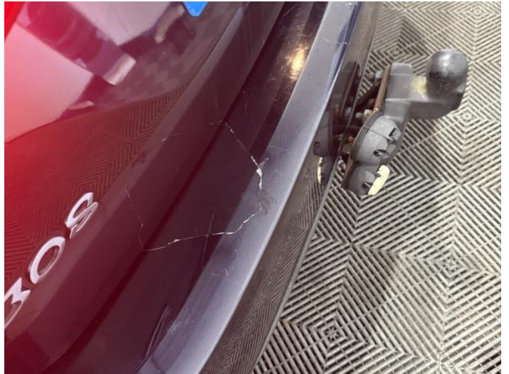
10: Bumper Rear Poor Previous Repair Paint Flake
