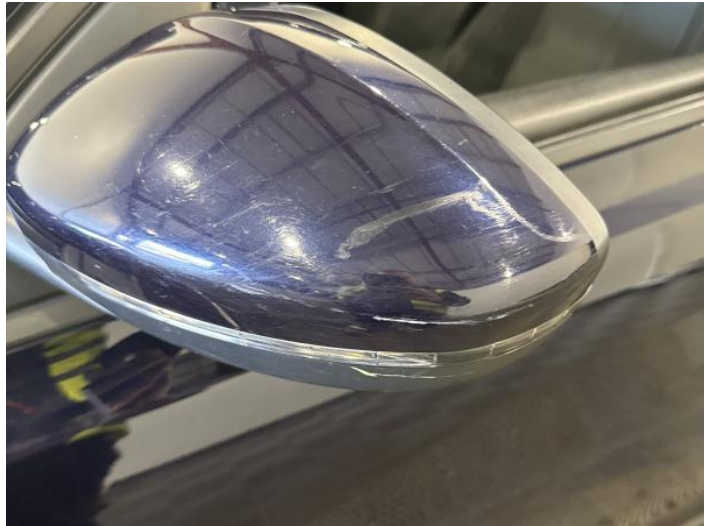
4: Door Mirror Assy nsf Scratched (Painted) Over 25mm Thru Paint
