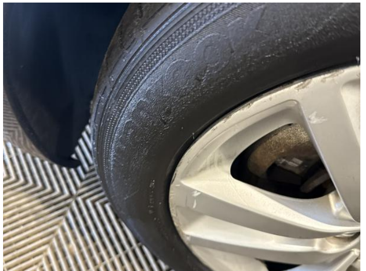
12: Tyre nsf Damaged Replace
