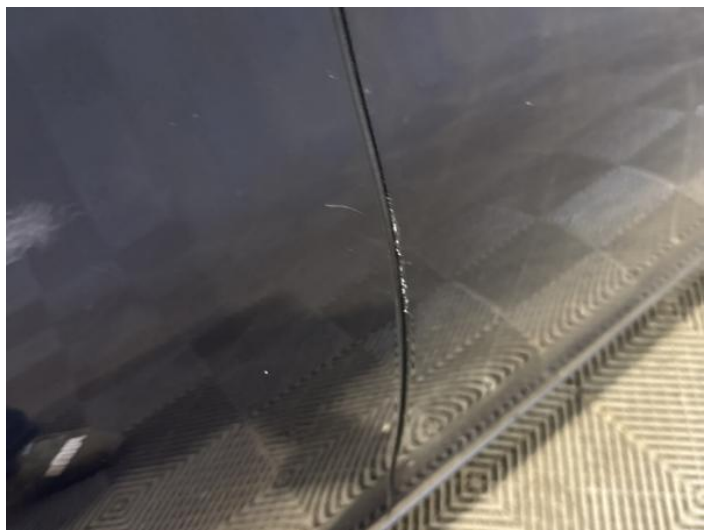
14: Door osr Scratched UpTo 25mm Thru Paint
