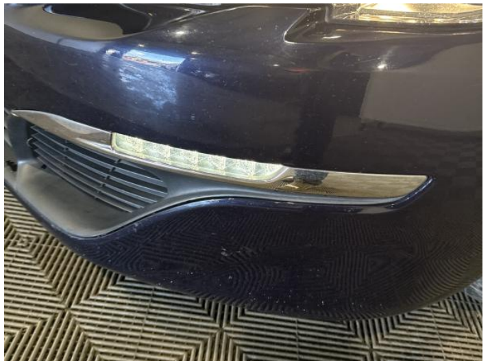
2: Bumper Front Chipped Multiple Chips
