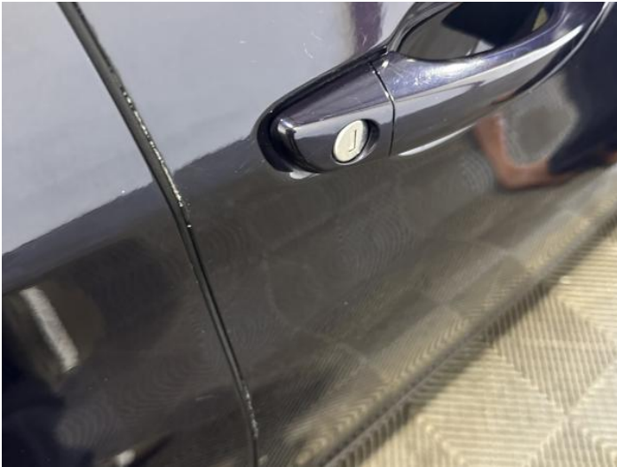
15: Door osf Chipped Edge Chip
