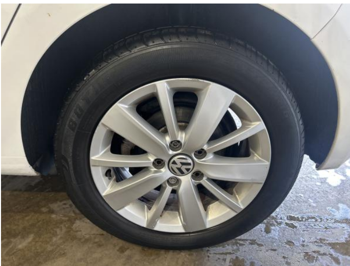
7: Wheel nsr Scratched Over 50mm
