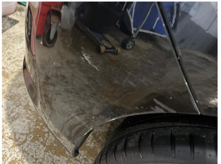
6: Bumper Rear Scratched Over 100mm Thru Paint
