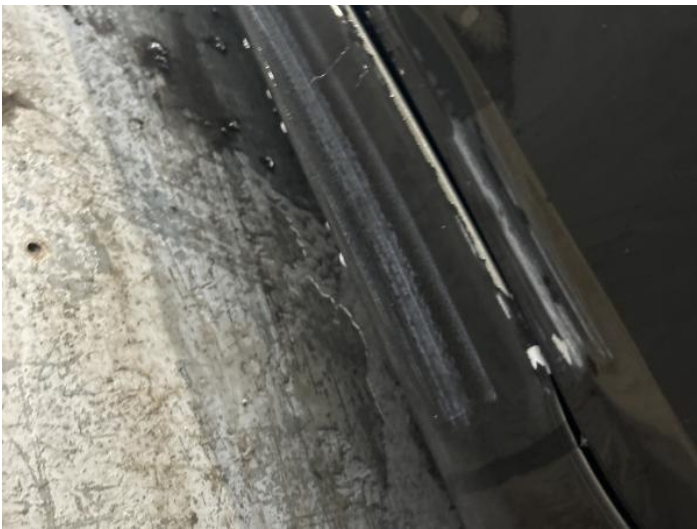
11: Sill ns Dented With Paint Damage
