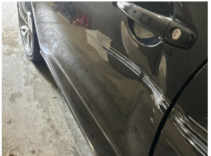
12: Door nsf Dented Over 30% Of Panel
