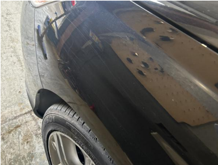
15: Wing nsf Scratched Over 25mm Not Thru Paint
