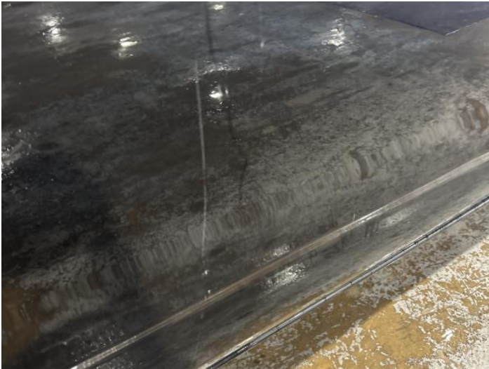
3: Door osf Scratched Over 25mm Thru Paint
