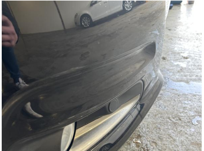
16: Bumper Front Scratched Over 100mm Thru Paint
