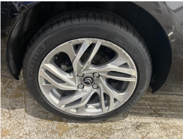
5: Wheel osr Corroded Light
