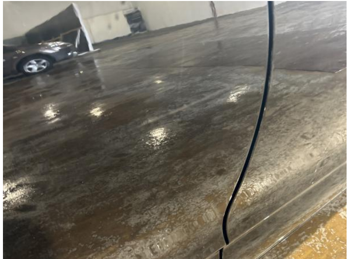
4: Door osr Scratched Over 25mm Thru Paint
