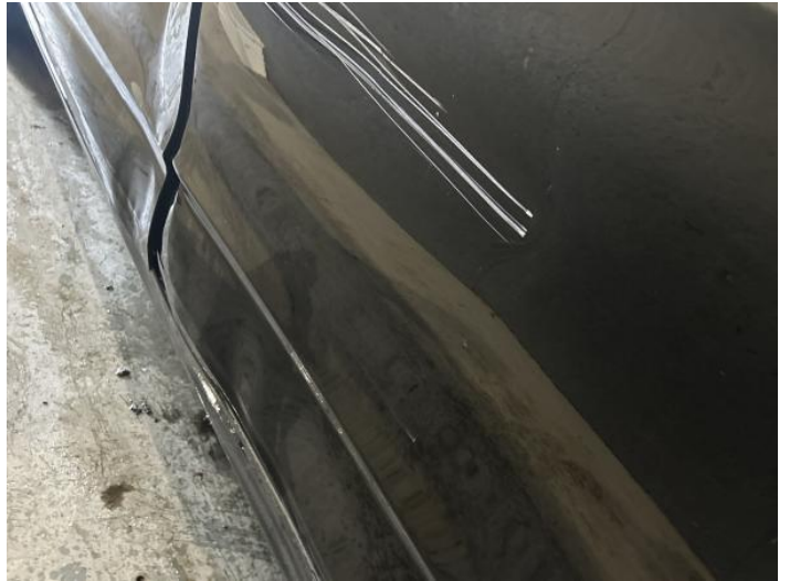
10: Door nsr Dented Over 30% Of Panel
