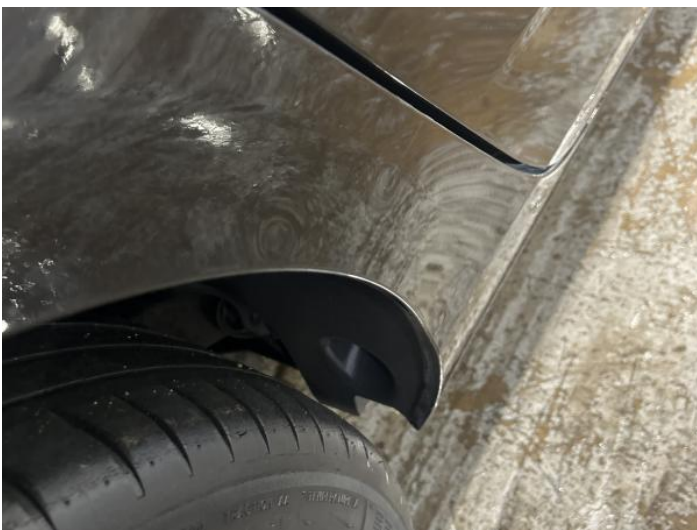
7: Qtr Panel osr Dented Over 2 UpTo 10mm
