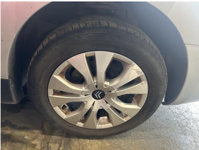
1: Wheel osf Scratched Over 50mm
