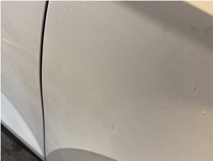
9: Wing osf Dented With Paint Damage
