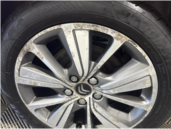
9: Wheel nsr Scratched Over 50mm
