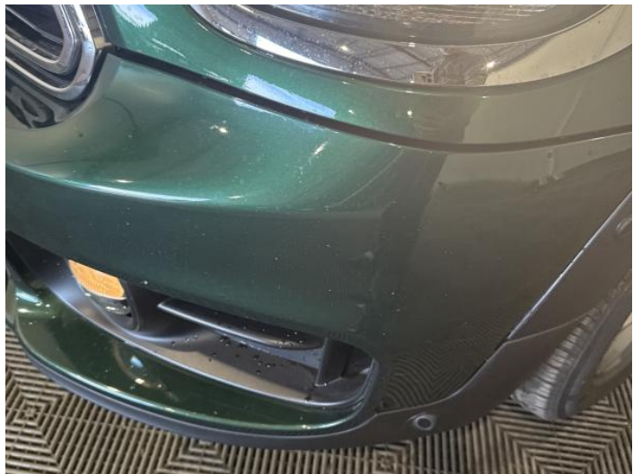
2: Bumper Front Scratched 25 to 100mm Thru Paint
