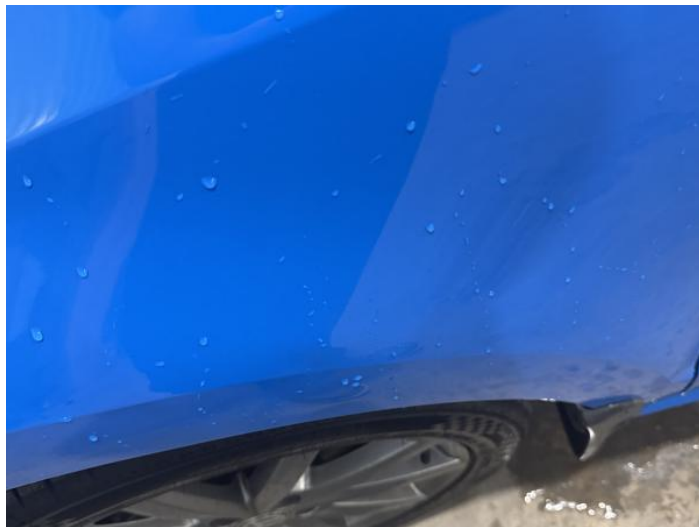
4: Wing nsf Dented Over 2 UpTo 10mm
