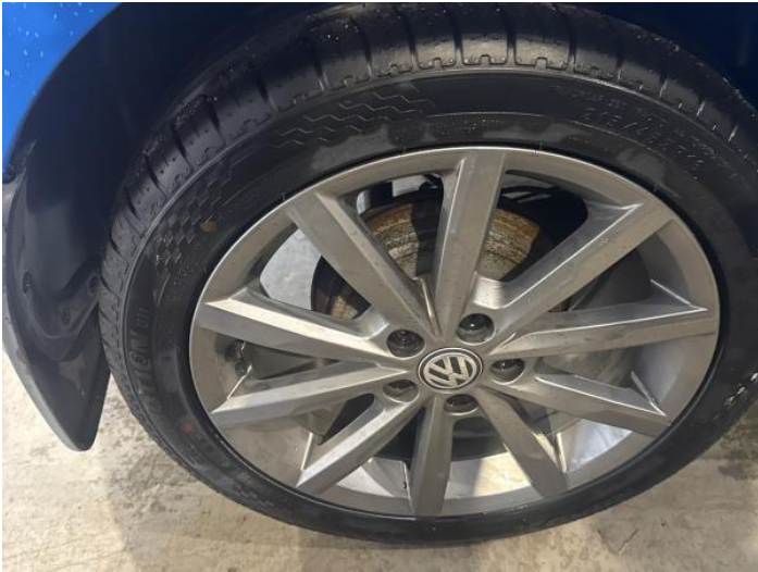
9: Wheel osr Scratched Up To 50mm
