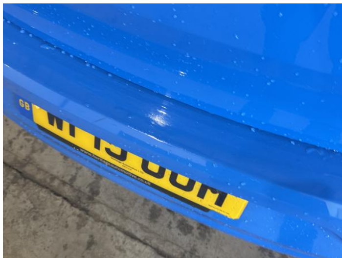
8: Bumper Rear Scratched 25 to 100mm Thru Paint
