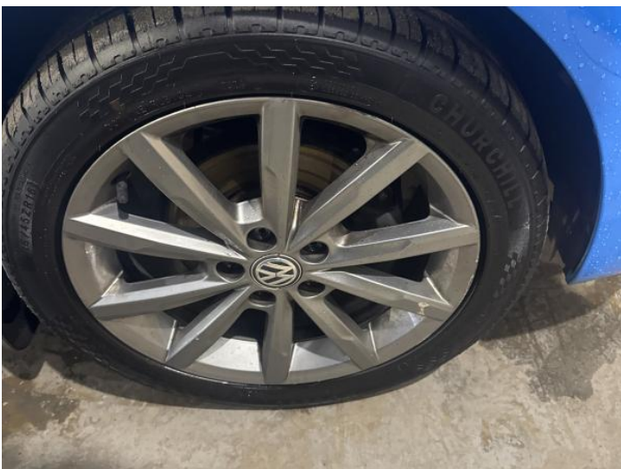
13: Wheel osf Scratched Over 50mm
