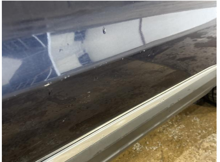
4: Door osf Chipped Multiple Chips
