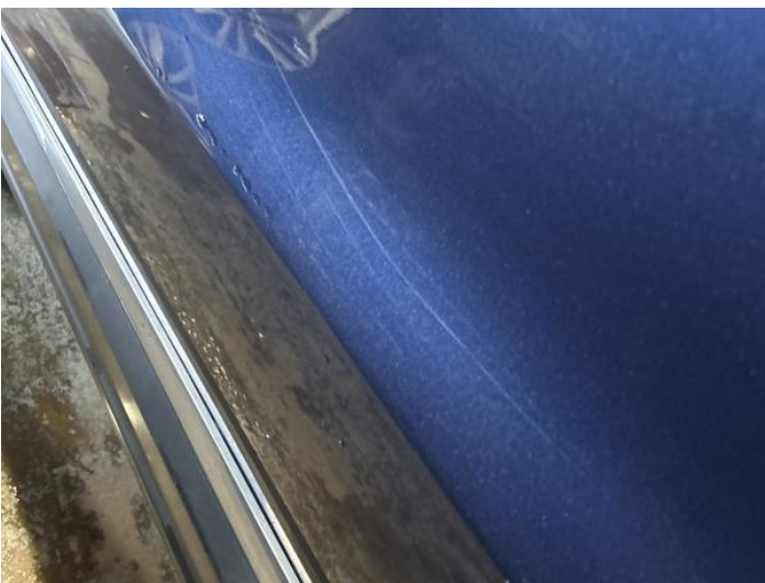
13: Door nsf Scratched Over 25mm Not Thru Paint
