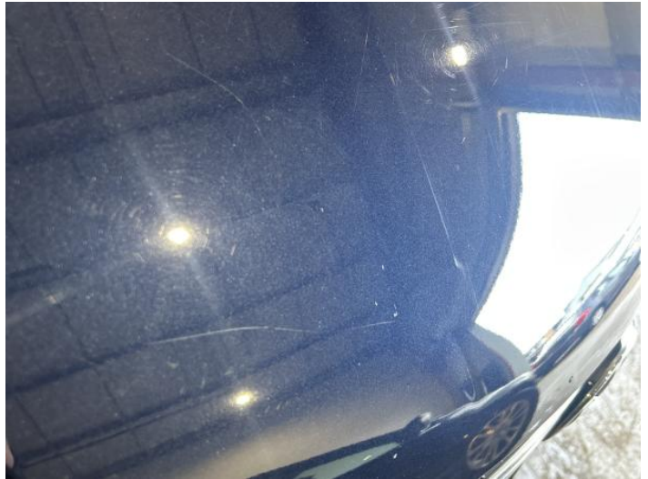
16: Bonnet Scratched Over 25mm Thru Paint
