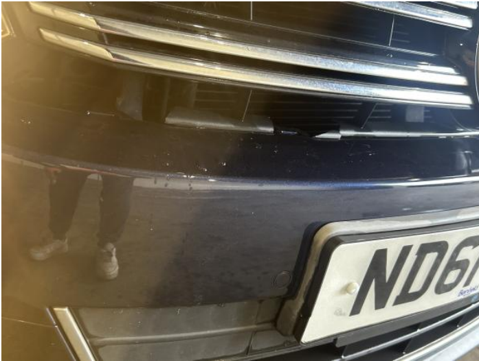
15: Bumper Front Grill Broken Replace
