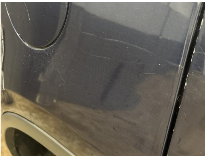
7: Qtr Panel osr Scratched Over 25mm Not Thru Paint
