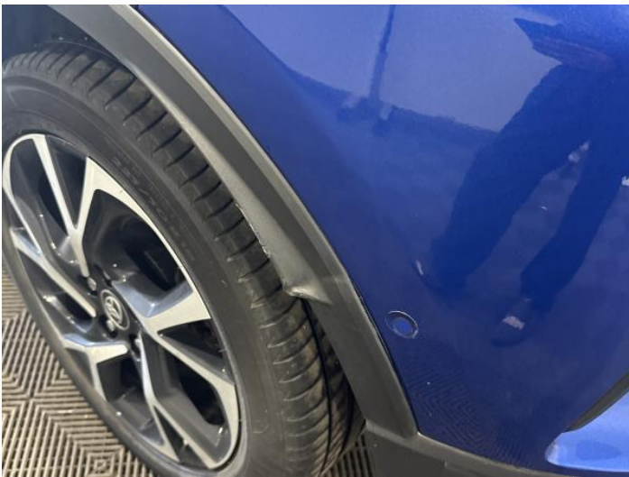
5: Qtr Panel Arch Extension ns Scuffed (Unpainted) Over 100mm
