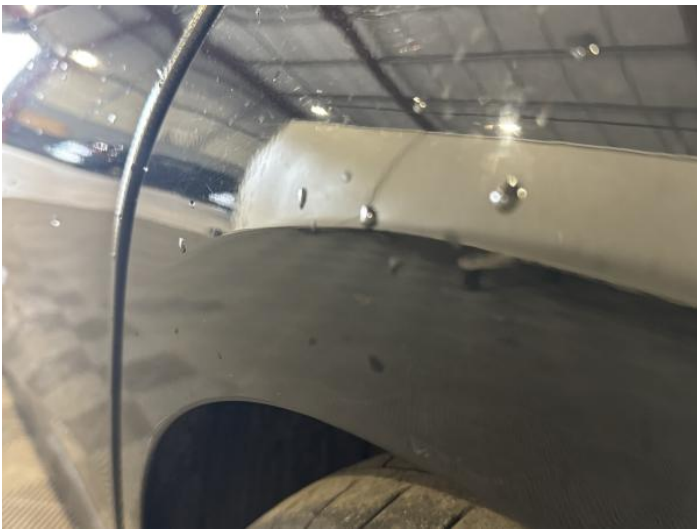
5: Qtr Panel nsr Dented Over 30mm
