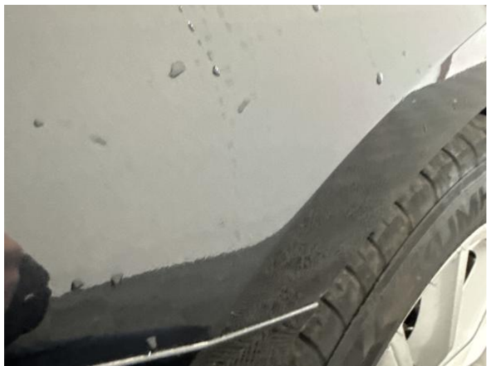
8: Qtr Panel osr Chipped 1 To 5
