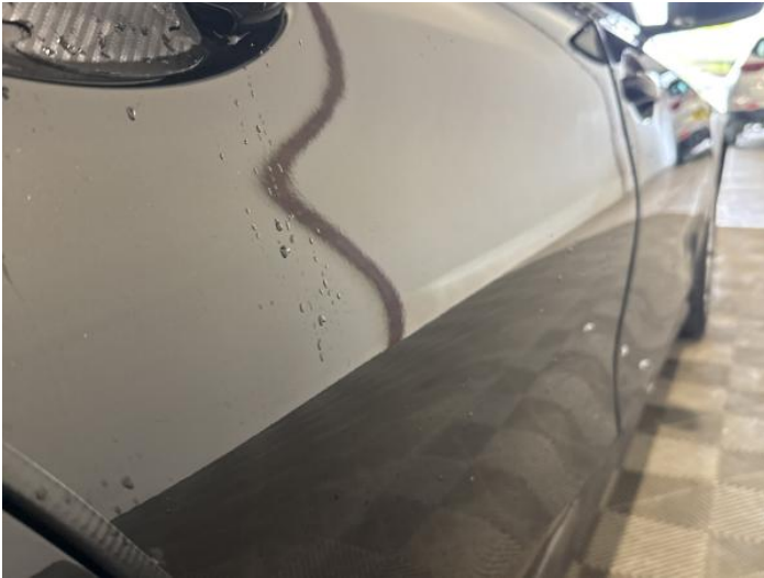
9: Door osr Poor Previous Repair Rippled UpTo 30%
