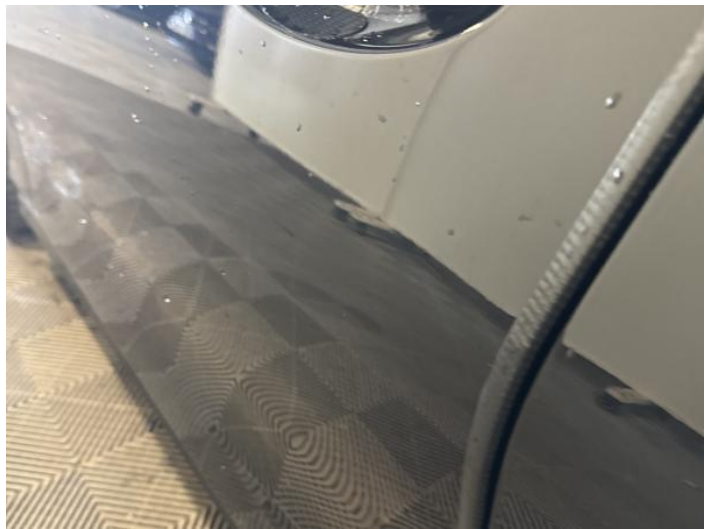
6: Door nsf Dented Between 10mm + 30mm
