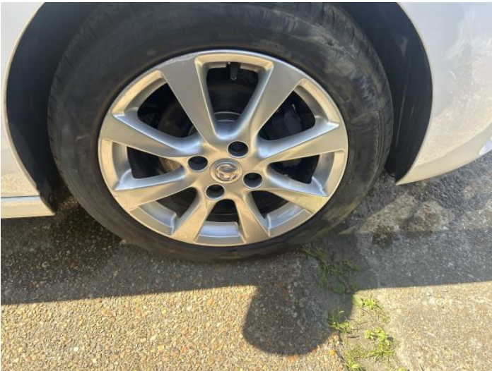
1: Wheel osf Scratched Over 50mm
