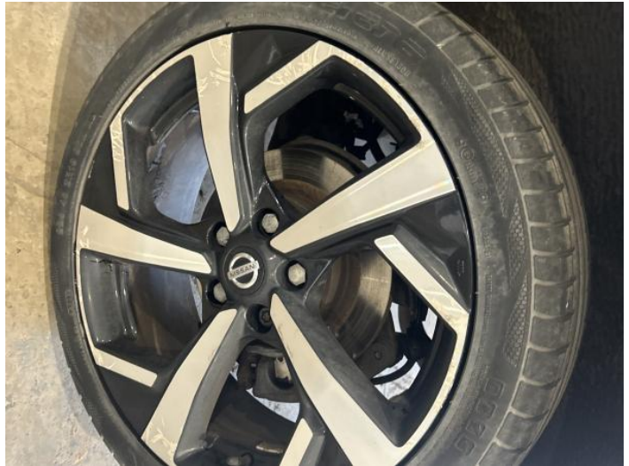
10: Wheel nsr Scratched Over 50mm
