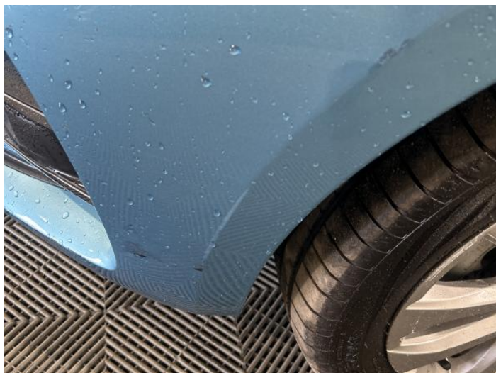
3: Bumper Front Scratched 25 to 100mm Thru Paint
