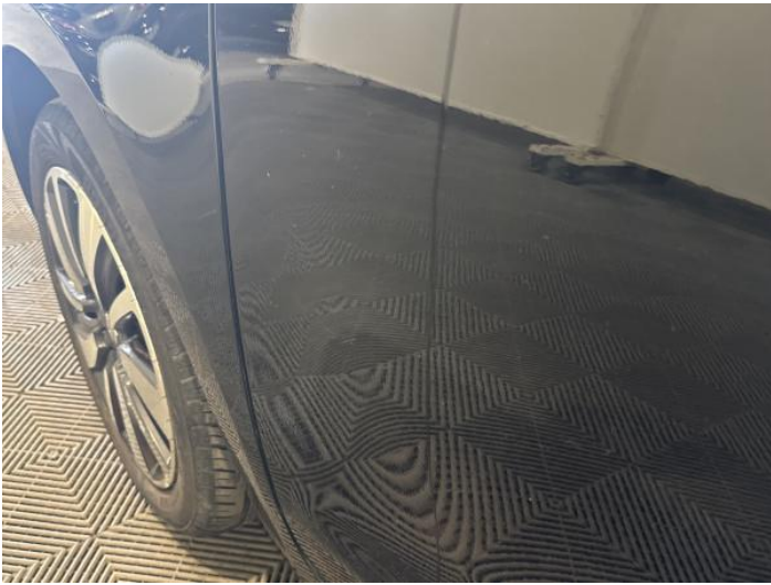
5: Door nsf Scratched Over 25mm Thru Paint
