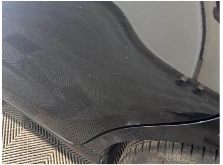
6: Door nsr Scratched UpTo 25mm Thru Paint
