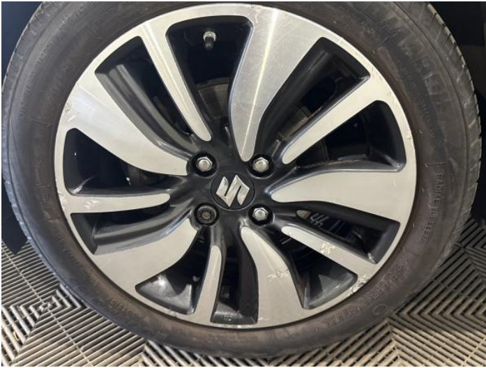
3: Wheel nsf Scratched Over 50mm
