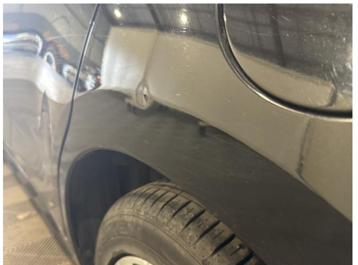
8: Qtr Panel nsr Dented Over 30mm
