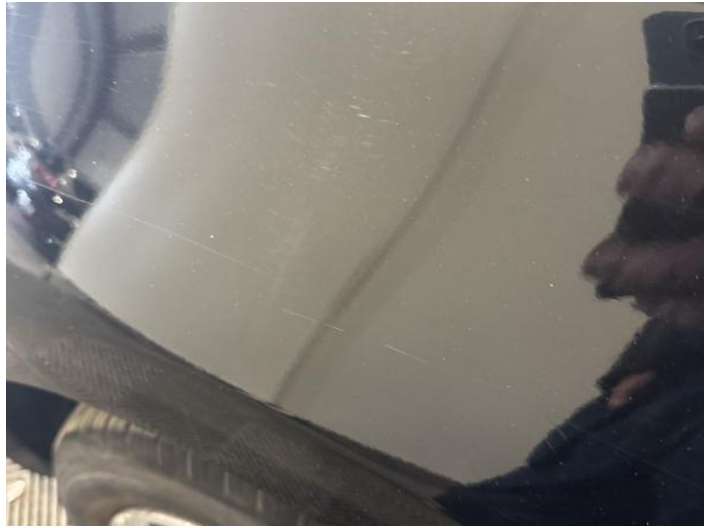
4: Wing nsf Scratched Over 25mm Thru Paint
