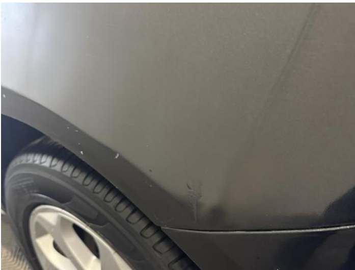
11: Qtr Panel nsr Poor Previous Repair Poor Paint
