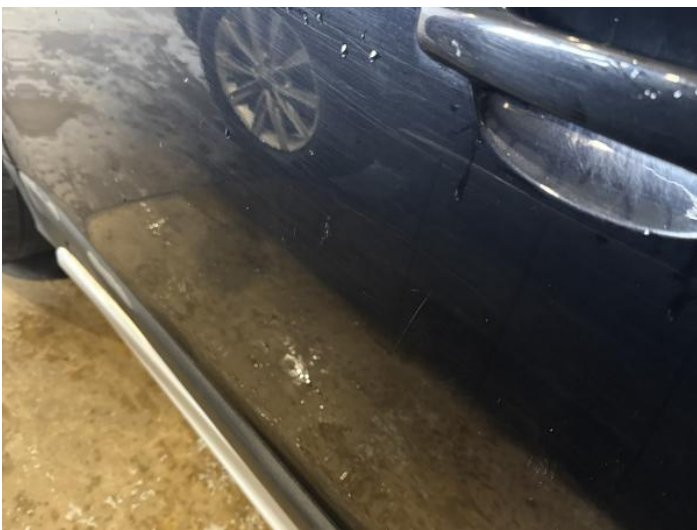
7: Door nsf Scratched Over 25mm Thru Paint
