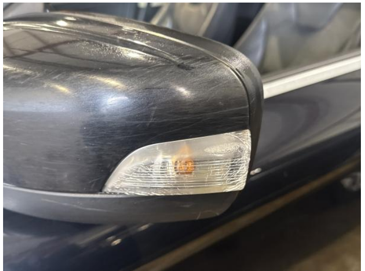
6: Flasher Side Repeater ns Broken Replace
