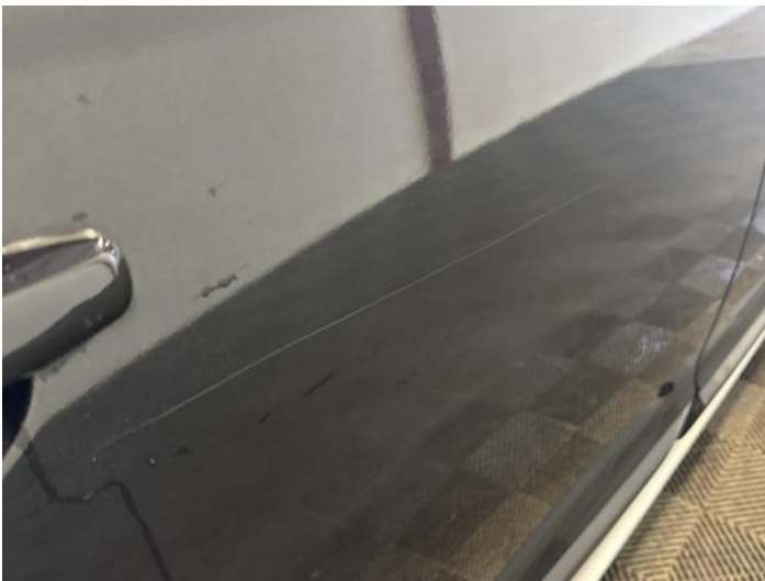
17: Door osf Scratched Over 25mm Thru Paint
