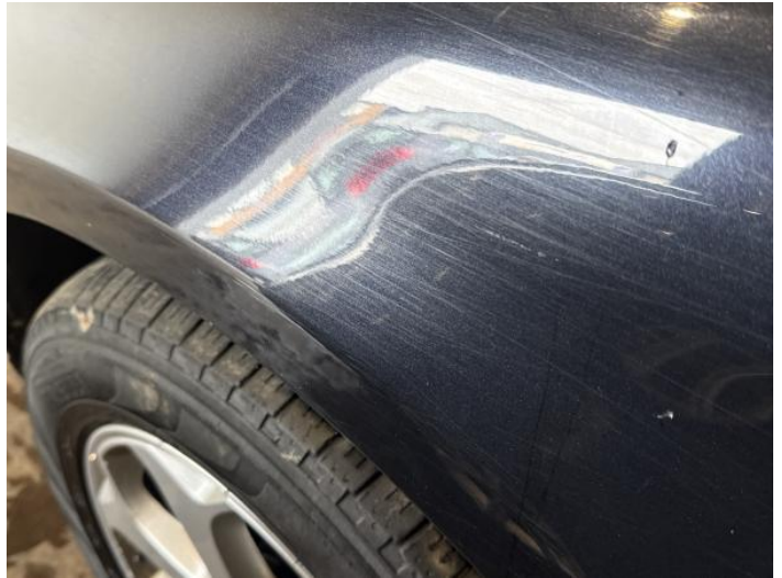
4: Wing nsf Scratched Over 25mm Thru Paint
