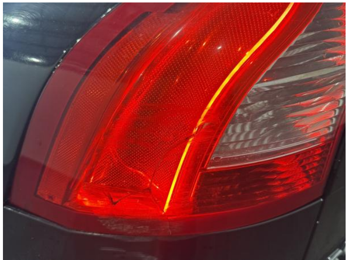
12: Lamp nsr Broken Replace
