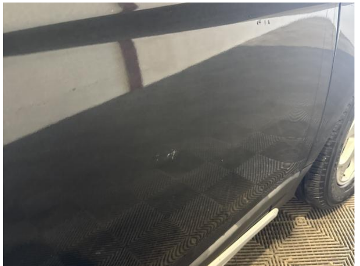
18: Door osf Scratched Over 25mm Thru Paint
