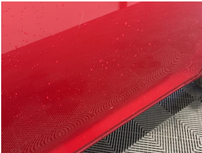
9: Door osf Scratched Over 25mm Not Thru Paint
