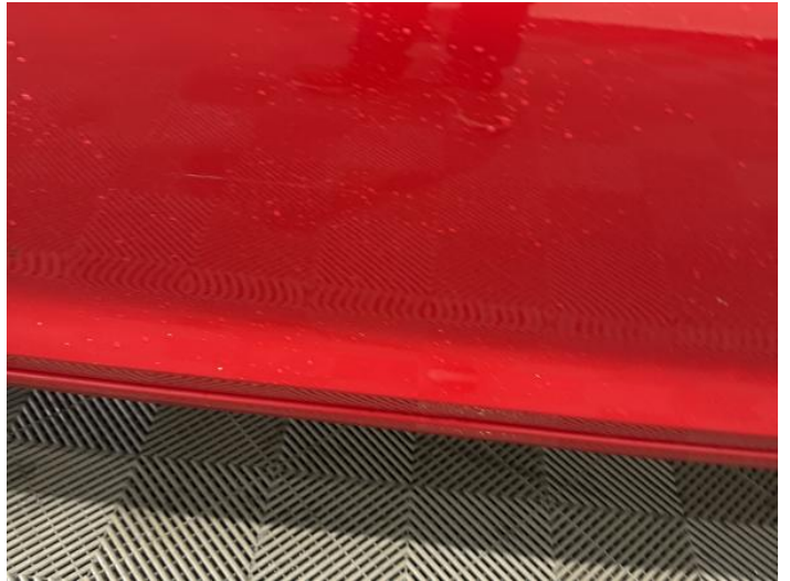
4: Door nsf Scratched Over 25mm Thru Paint
