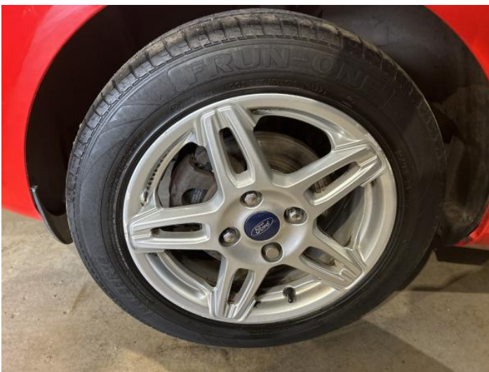
19: Wheel nsf Scratched Over 50mm
