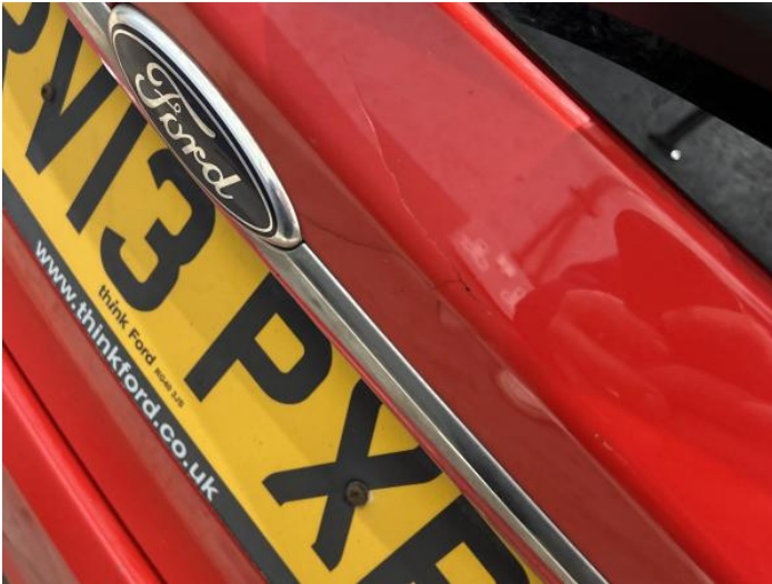
9: Tailgate Poor Previous Repair Poor Paint
