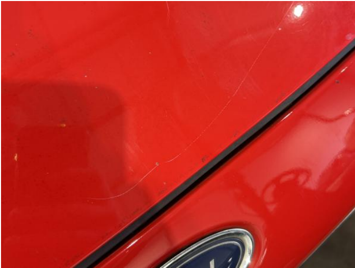
15: Bonnet Scratched Over 25mm Thru Paint
