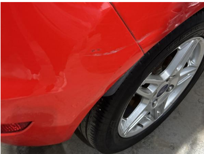
7: Bumper Rear Scratched 25 to 100mm Thru Paint
