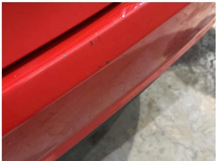
8: Bumper Rear Chipped Multiple Chips
