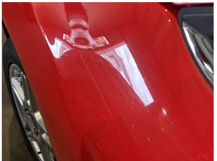
14: Wing nsf Scratched Over 25mm Not Thru Paint
