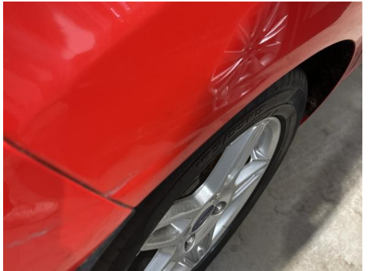
6: Qtr Panel osr Dented With Paint Damage
