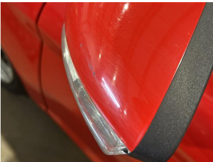
13: Door Mirror Assy nsf Scratched (Painted) Up To 25mm Thru Paint
