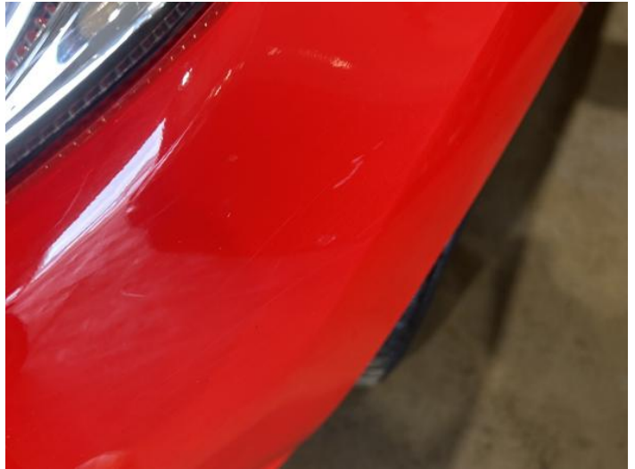
16: Bumper Front Scratched Over 25mm Not Thru Paint
