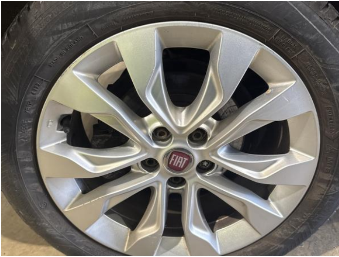
15: Wheel osr Scratched Up To 50mm
