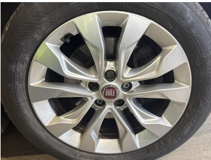
19: Wheel osf Scratched Over 50mm
