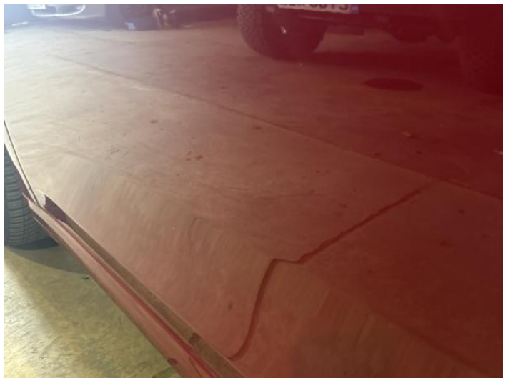
6: Door nsf Dented Between 10mm + 30mm
