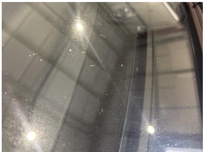
20: Screen Front Chipped UpTo 10mm
