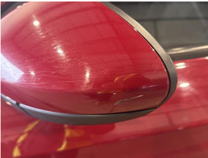
5: Door Mirror Assy nsf Scratched (Painted) Over 25mm Thru Paint
