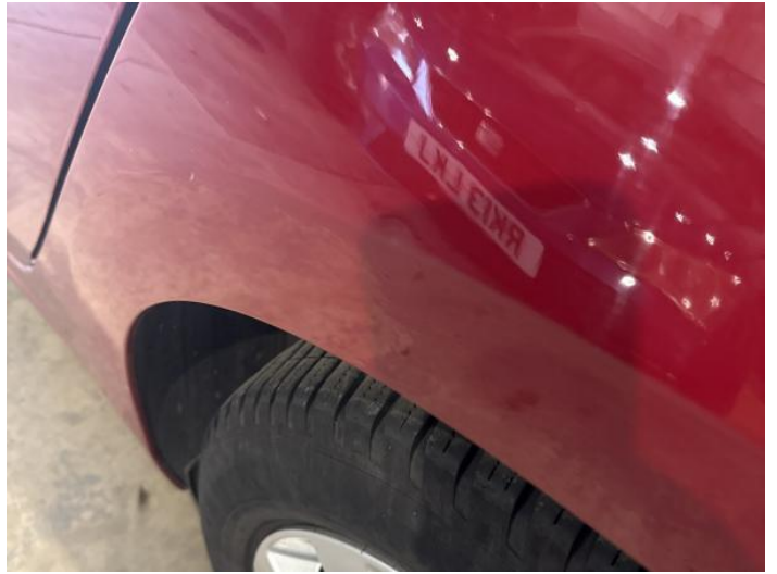
10: Qtr Panel nsr Dented Between 10mm + 30mm
