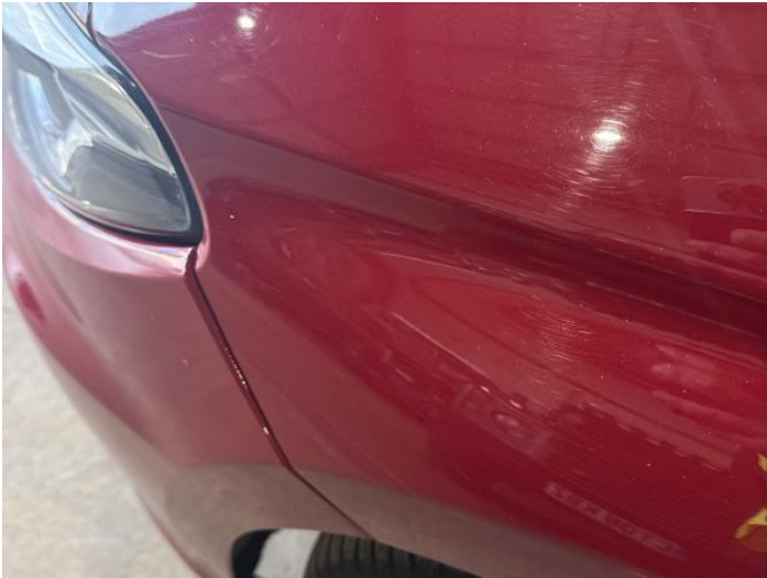
3: Wing nsf Scratched Over 25mm Thru Paint
