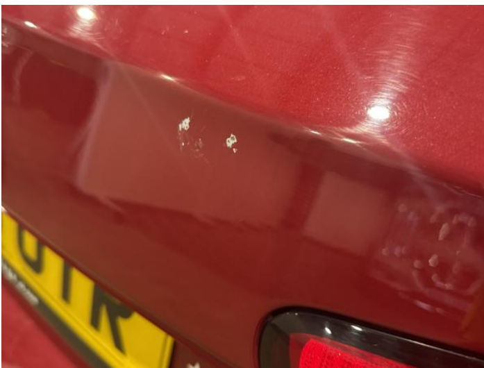
13: Tailgate Scratched Over 25mm Thru Paint
