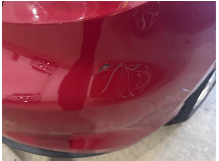
12: Bumper Rear Dented With Paint Damage
