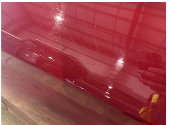
8: Door nsr Scratched Over 25mm Thru Paint
