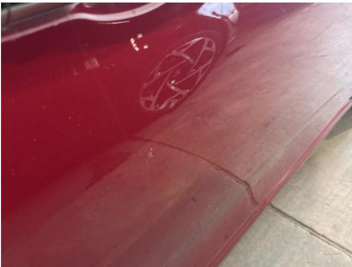
17: Door osf Dented Over 30mm
