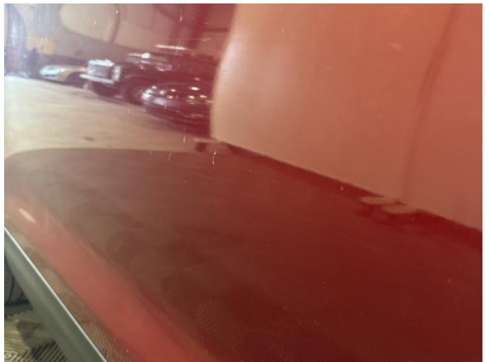
6: Door nsf Scratched Over 25mm Thru Paint
