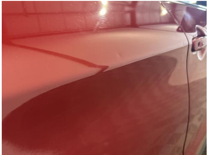
12: Door osr Dented Between 10mm + 30mm
