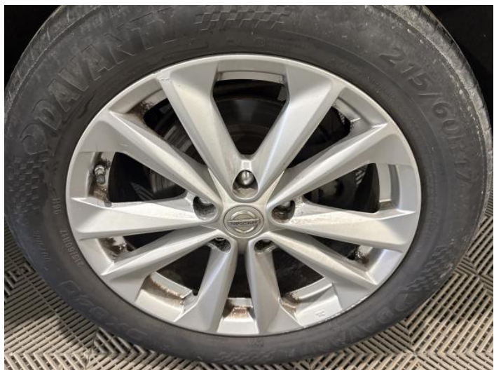
8: Wheel nsr Corroded Light
