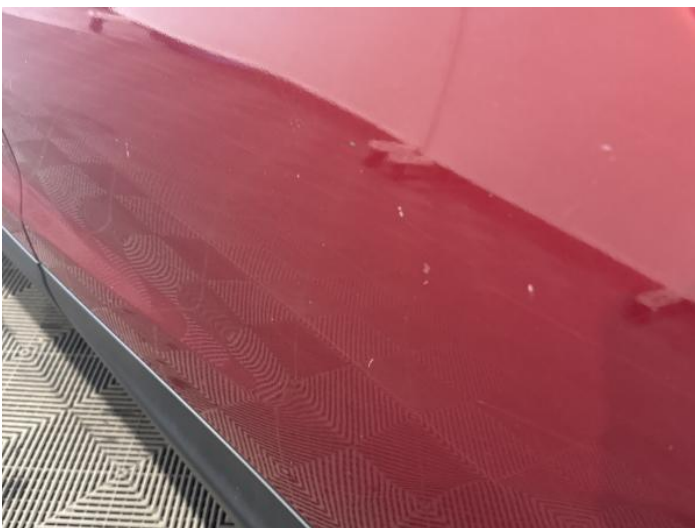
7: Door nsr Scratched Over 25mm Thru Paint
