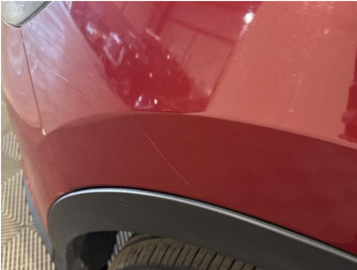
3: Wing nsf Scratched Over 25mm Thru Paint
