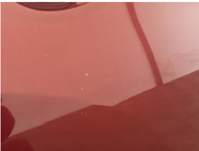
13: Door osr Chipped 1 To 5
