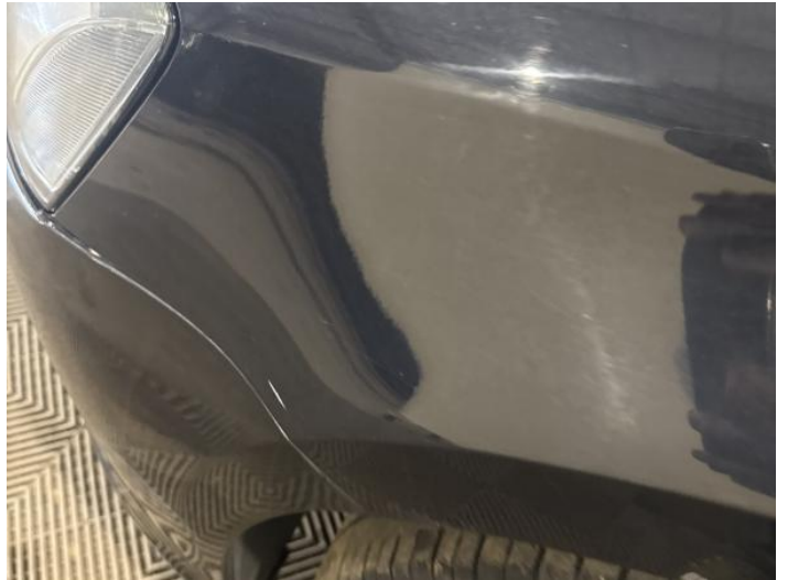
4: Wing nsf Scratched UpTo 25mm Thru Paint
