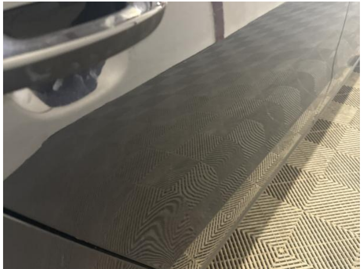
12: Door osf Dented Over 30mm
