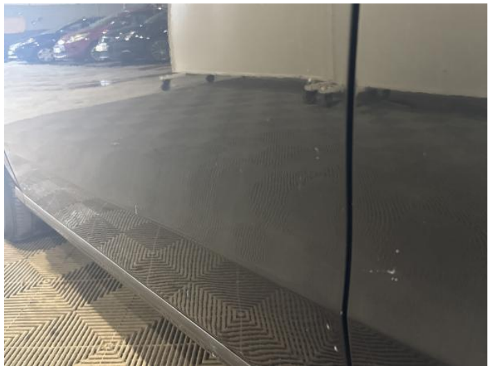
6: Door nsf Scratched Over 25mm Thru Paint
