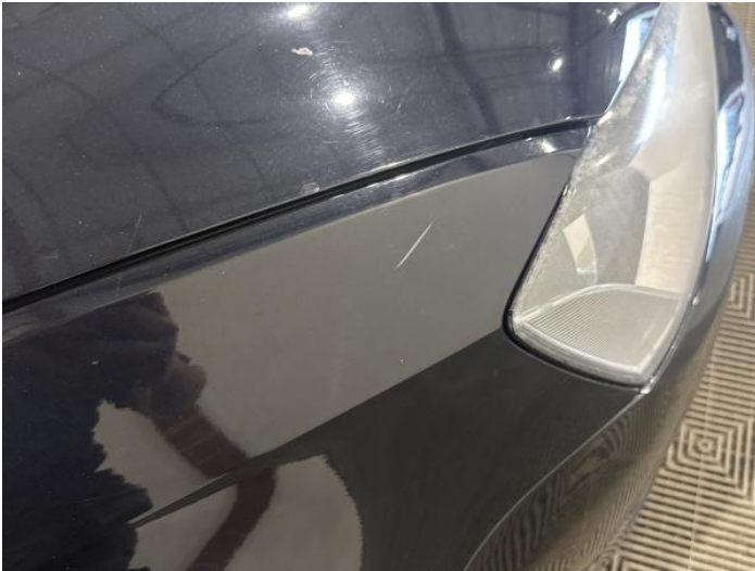
15: Wing osf Scratched Over 25mm Thru Paint
