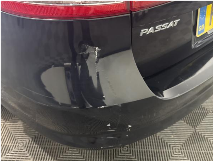
9: Bumper Rear Cracked UpTo 25mm
