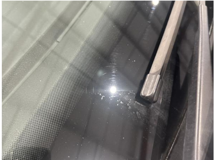
16: Screen Front Chipped UpTo 10mm
