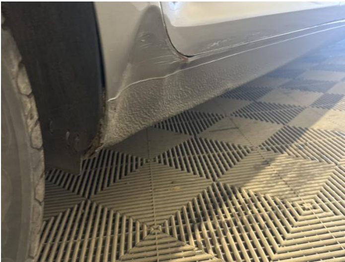
11: Sill os Dented With Paint Damage
