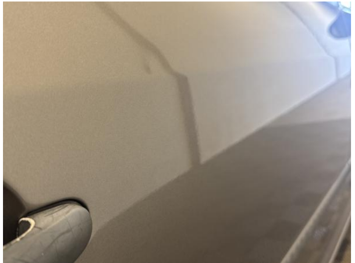
12: Door osr Dented Between 10mm + 30mm
