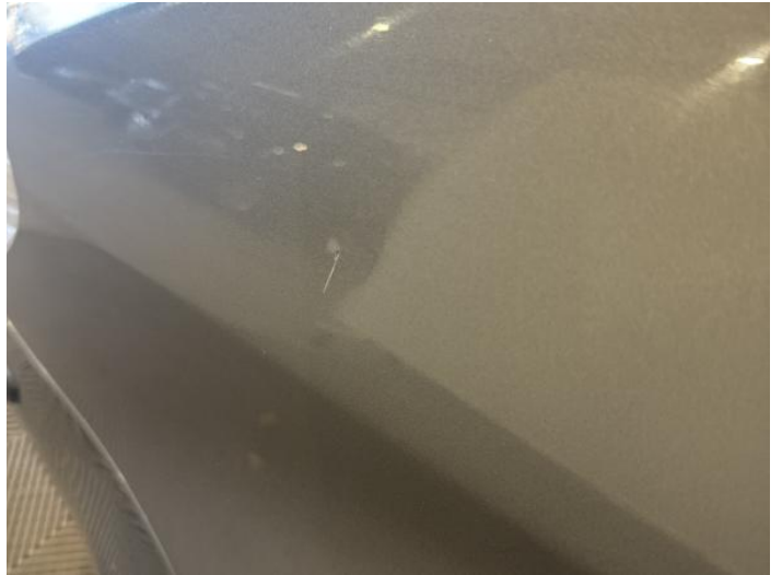
4: Wing nsf Scratched UpTo 25mm Thru Paint
