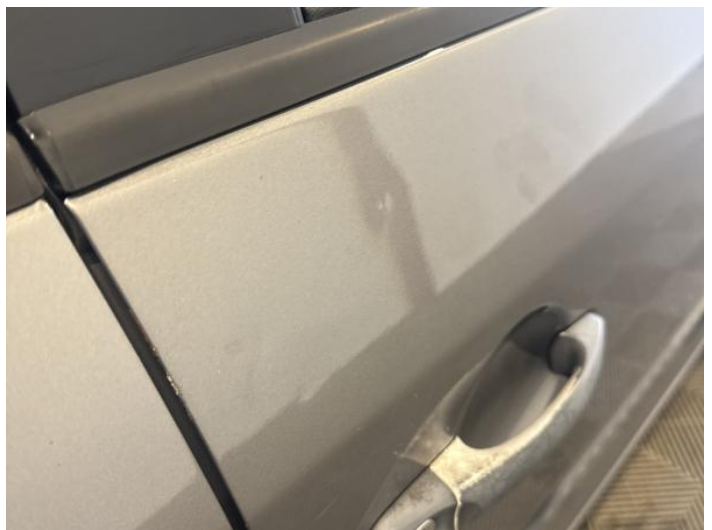
14: Door osf Dented Between 10mm + 30mm
