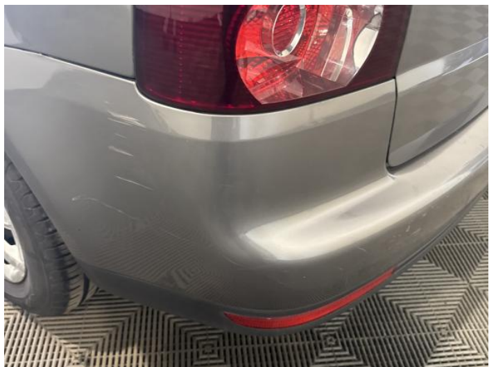
8: Bumper Rear Scratched Over 100mm Thru Paint
