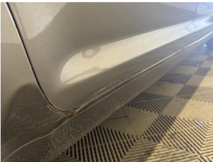
13: Door osr Scratched Over 25mm Thru Paint
