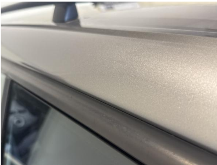
17: B Post os Dented Between 10mm + 30mm
