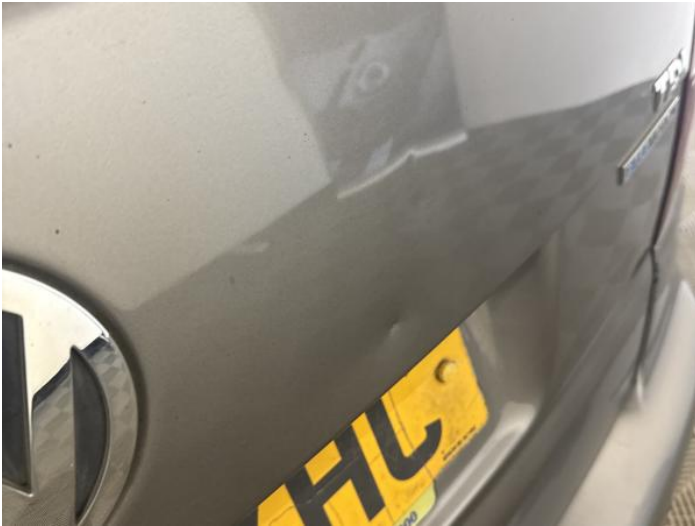
9: Tailgate Dented Over 30mm
