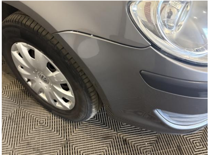
16: Bumper Front Insecure Action Required
