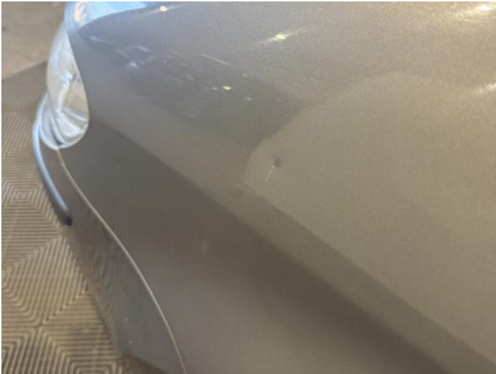
3: Wing nsf Dented Between 10mm + 30mm
