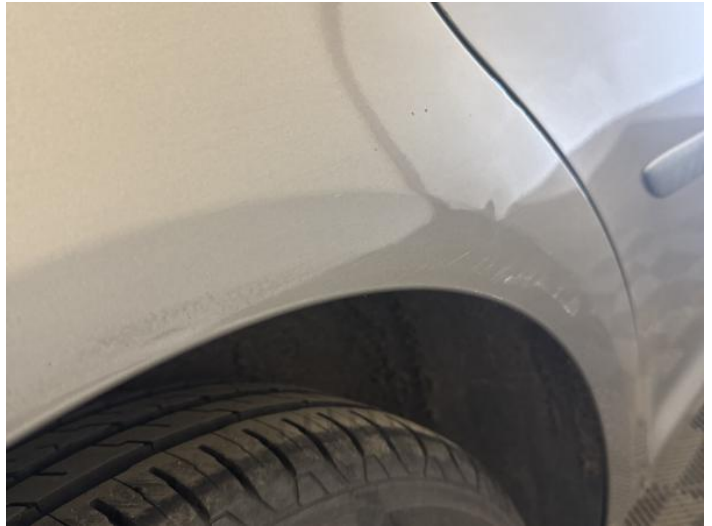
10: Qtr Panel osr Dented With Paint Damage
