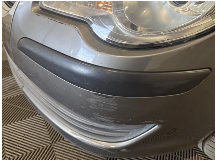
2: Bumper Front Scratched Over 100mm Thru Paint
