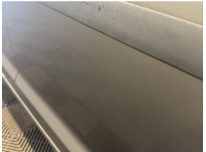
6: Door nsr Scratched Over 25mm Thru Paint
